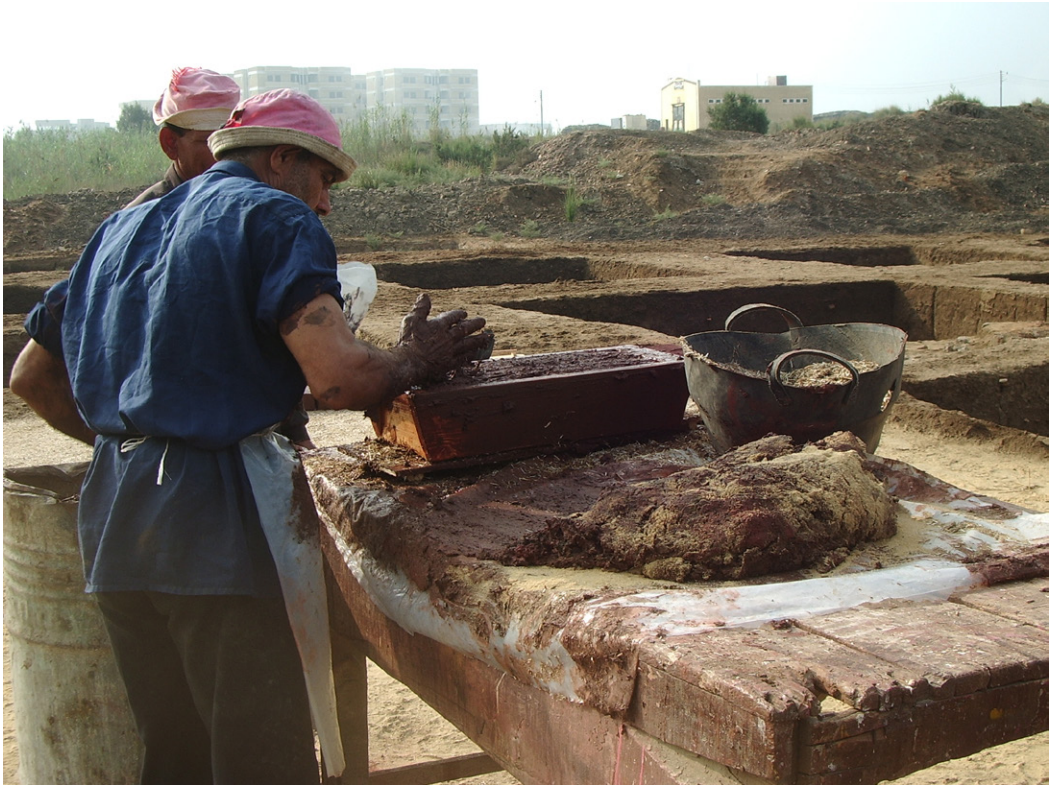
Figure 8. Moulding of the mudbricks (M. Lorenzon).
