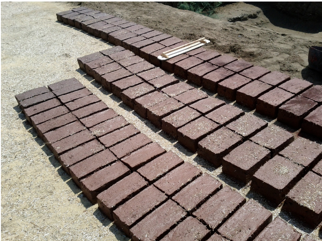
Figure 9. Mudbricks left to dry, with a wooden finishing trowel used to smooth the upper surface (Photo credit: Sarah Hitchens).
