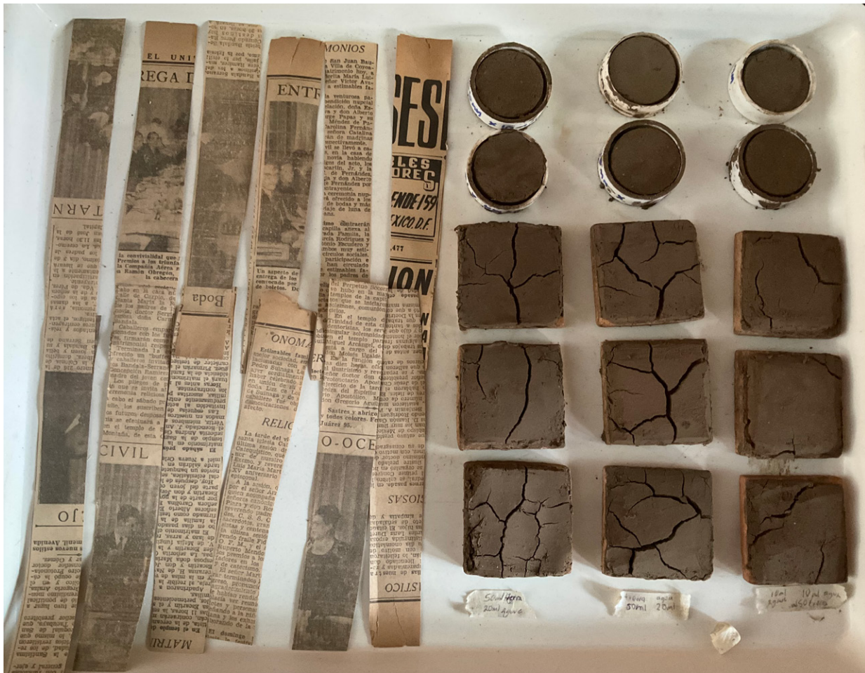
Figure 4. Tests with orchid mucilage used as a glue for paper and as an aggregate for earthen coatings in different proportions.
