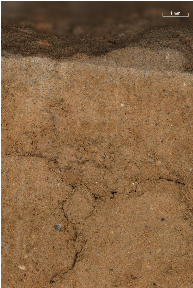
Figure 7. Section of a fragment from Gröbitz. No separate layers, such as a white finish or paint, are visible under the microscope. In fact, the matrix becomes lighter towards the surface, but it is still the same pure sandy loess (© LDA Saxony-Anhalt, C.-H. Wunderlich).
