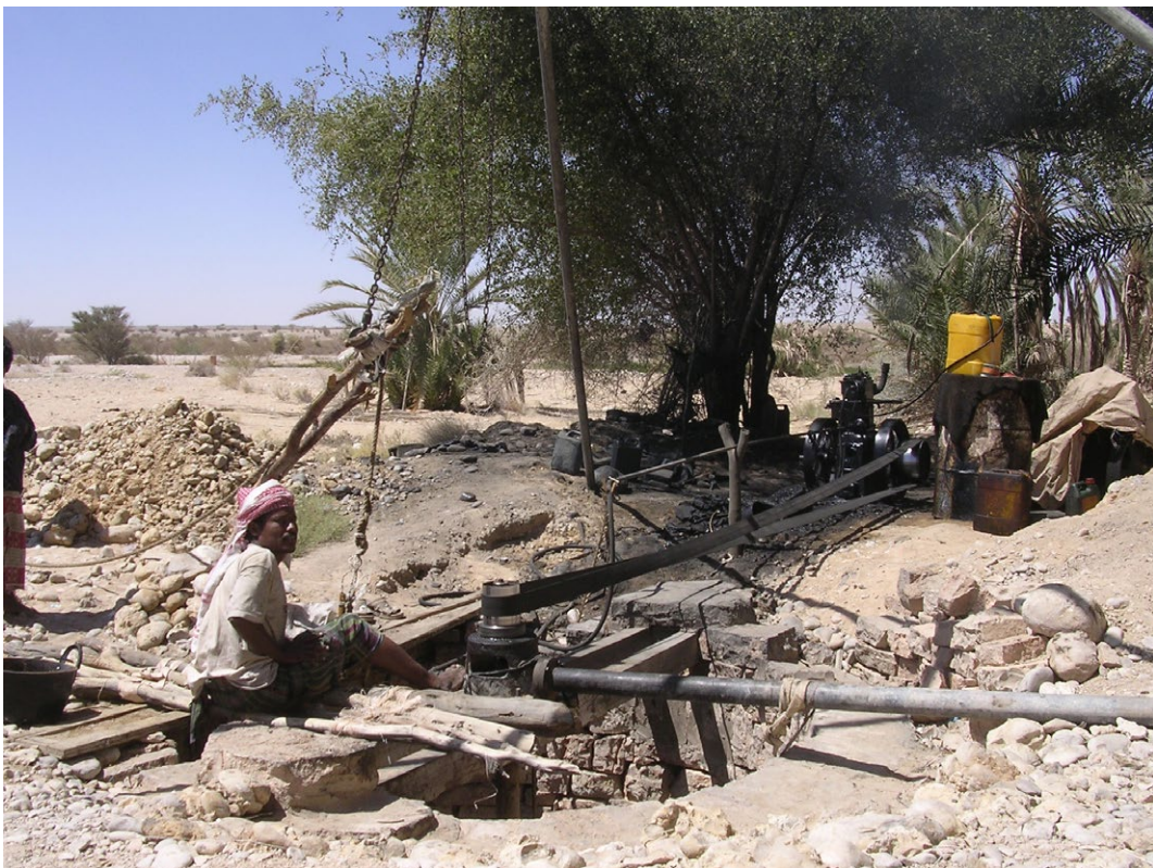
Figure 4. Water being drawn from a hand-dug well ( bi'r ) using a diesel pump in Ghayl Bin Yumain, Hadramawt, Yemen (photo. M. Harrower, 2005).
