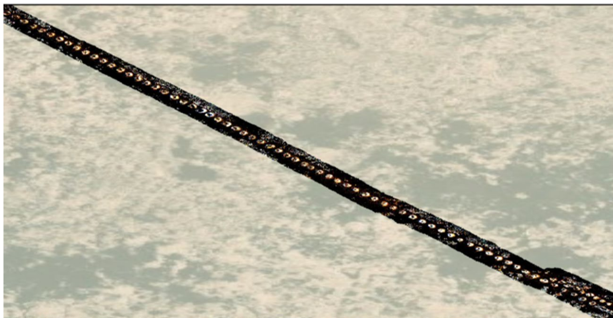
Figure 5. Aerial image showing the extension of the water channel, featuring the closely spaced openings known as Kharaz .
