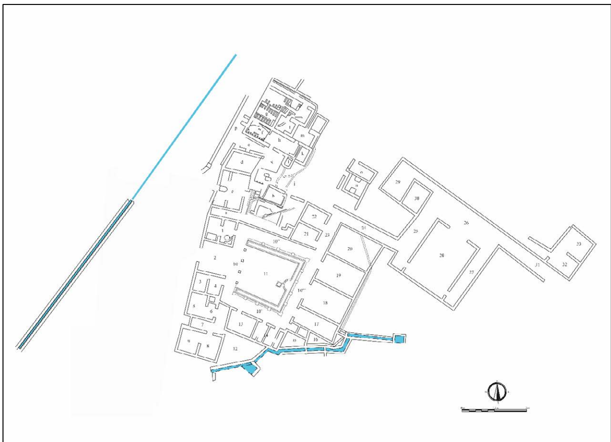
Figure 2. Plan of the House of the Amphitheatre in its early Roman phase indicating the aqueduct and the erogatio conduit (elab. by the authors).
