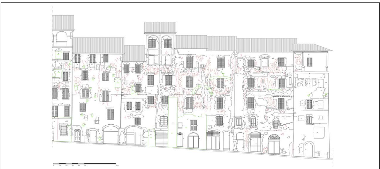
Figure 4.14 - Stratigraphic analysis of a portion of the street front in Via Pendola containing: stratigraphy (black colour), crack pattern (red colour), post-seismic construction techniques (green colour) Elaboration: Marco Repole.
