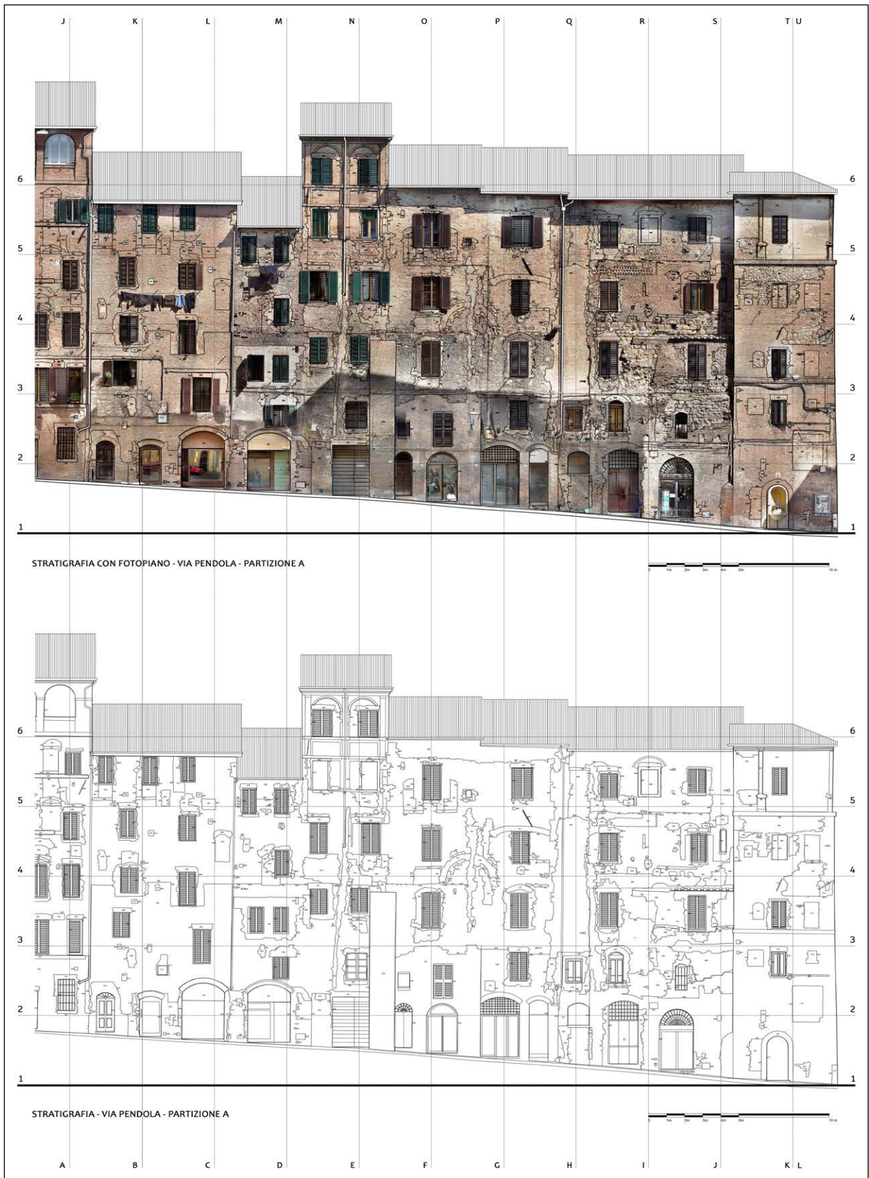
Figure 4.17b - Orthophoto plan (top) and stratigraphic analysis (bottom) of the east street front of Via Pendola.
