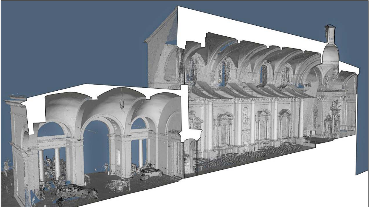
Figure 3.2 - Longitudinal section of the three-dimensional model of the Church of St. Augustine obtained by laser scanner and photogrammetric survey (elaboration: Marco Repole).
