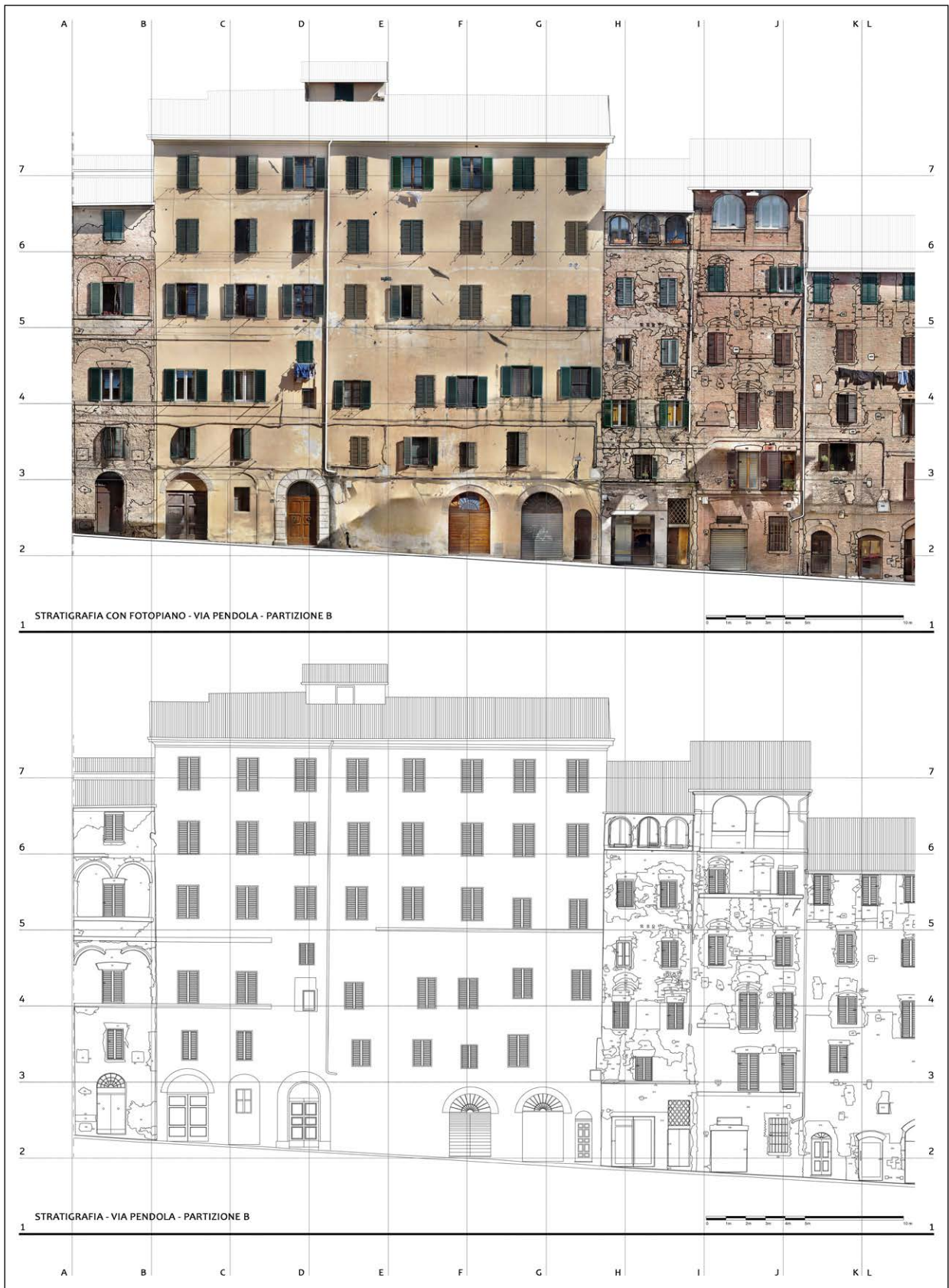
Figure 4.17a - Orthophoto plan (top) and stratigraphic analysis (bottom) of the west street front of Via Pendola.
