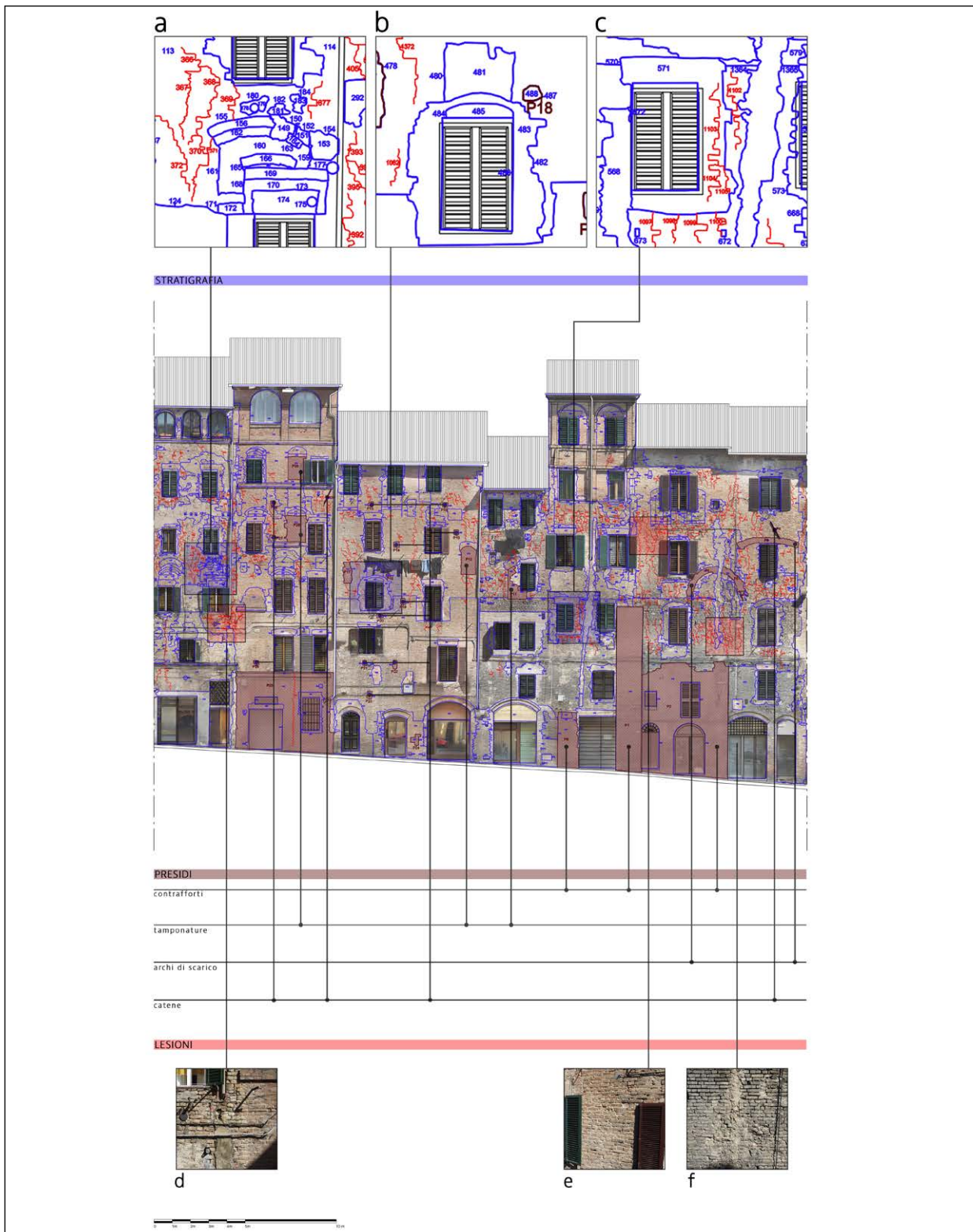
Figure 3.8 - Methodological table illustrating the digitization of the archaeological analyses carried out on the street front of Via Pendola. In the centre of the image is shown a photo-plan of a portion of the street front where the stratigraphic analysis, the characterization of the cracking framework and the documentation of the post-seismic techniques were carried out. Above are shown portions of the elevation (a, b, c) with enlargements of the stratigraphic analysis (in blue) and of the cracks pattern (in red). At the bottom, the post-seismic techniques and cracks are shown (d, e, f) (Elaboration: Marco Repole).
