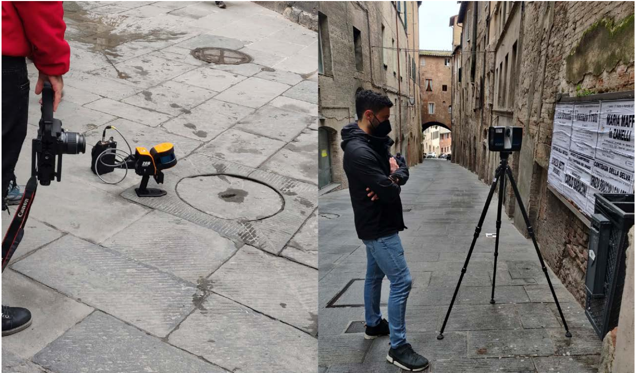
Figure 3.4 - Images of the survey fieldwork carried out using mobile and terrestrial laser scanners.
