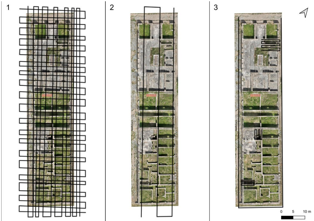
Figure 7 - Flights plan of the UAV survey.
