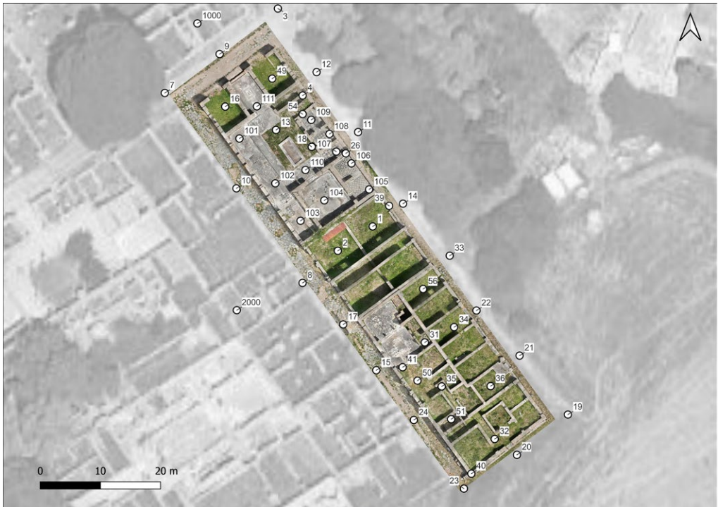
Figure 5 - Ground Control Points (GCP) located in block V, III (Google Earth base map, orthophoto from A. Peeters).
