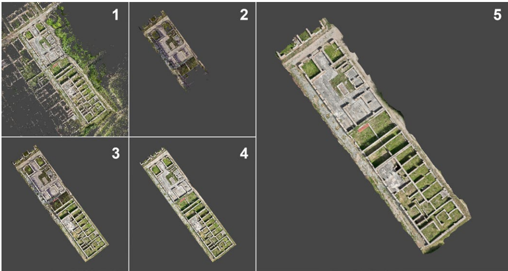
Figure 8 - The different steps in data processing and merging: (1) Photogrammetry image alignment; (2) TLS dense cloud; (3) Merging of TLS and photogrammetric dense clouds; (4) 3D Model; (5) Orthophoto.
