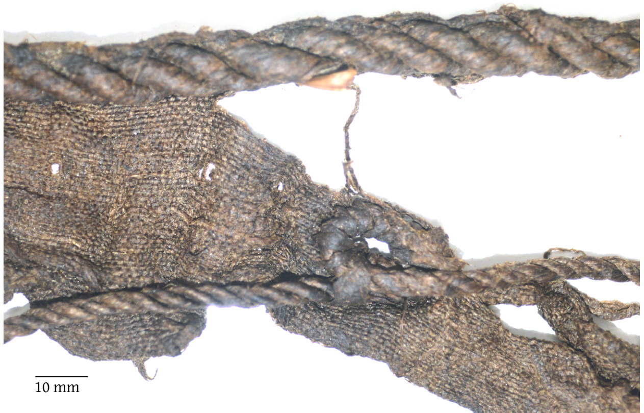
Figure 5.22. 1-inch rope and Roband stitched into the tabling
