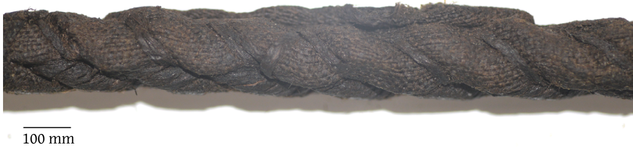
Figure 5.19. Sail cloth stitched to the boltrope
