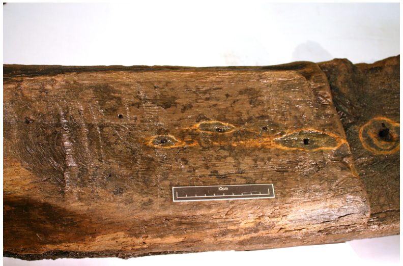
Figure 4.52. Axe marks on SCW1226
