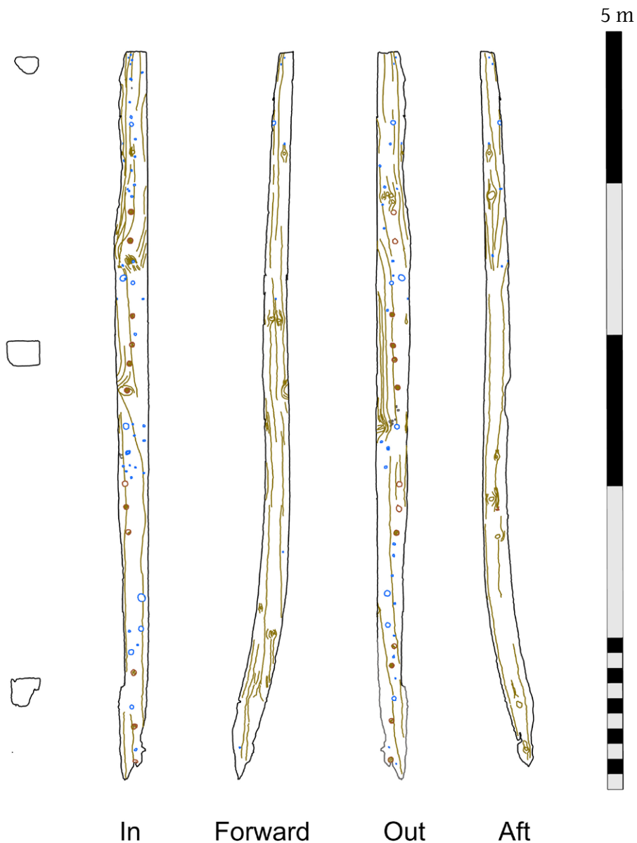
Figure 4.24. SCW1225 showing the curvature of the tumblehome
