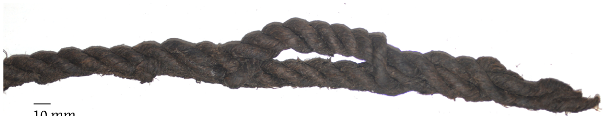
Figure 5.21. SCW989 cringle spliced into the leech-rope
