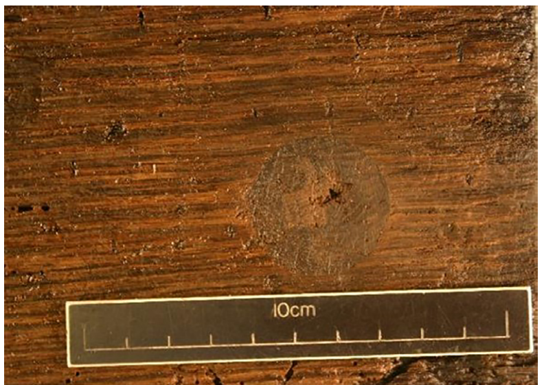
Figure 4.53. Treenail with square wooden pins present
