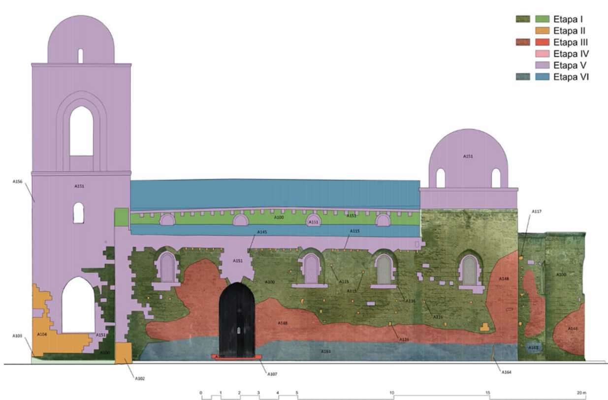
Figure 6 – Archaeological records of the south façade of San Giovanni
