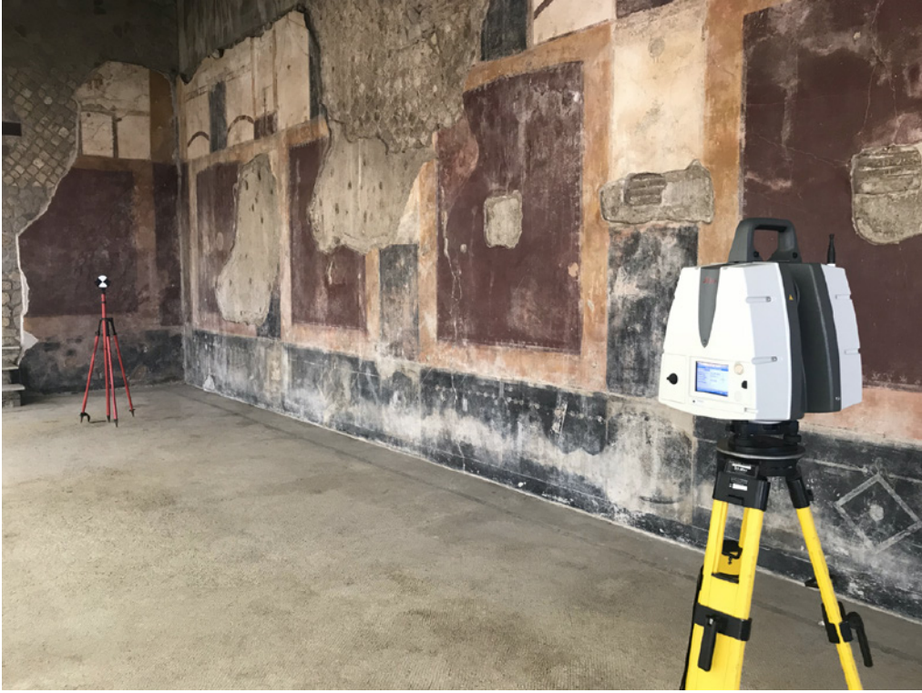
Figure 6. Castellammare di Stabia. Villa San Marco. Leica P30 laser scanner being acquired (photo by the author).
