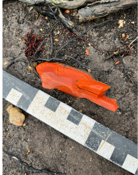
Unburnt propellant in and around the wreckage (credit: Falklands War Mapping Project)
