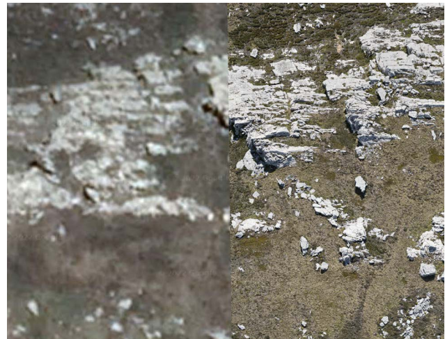
Comparison showing the high-resolution result of the drone-captured imagery (right) versus Google satellite imagery (left) (credit: Falklands War Mapping Project)
