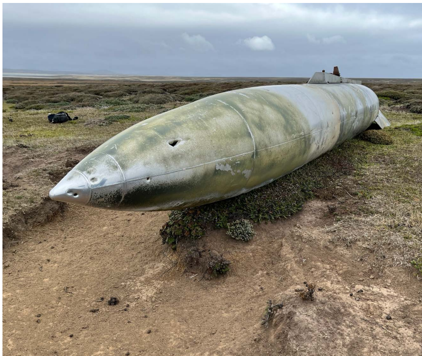
Jettisoned underwing fuel tank from Argentine dagger jet C-437 (credit: Falklands War Mapping Project)
