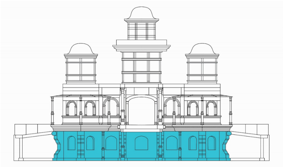
Figure 6. Frontal elevation of Lingzhao Xuan Pavilion with indications of the Sumeru-base in blue, rendered after a drawing in Fang Liyu, “The interdisciplinary research of virtual recovery and simulation of heritage buildings. Take Lingzhao Xuan in the Palace Museum as an example,” in Conservation Science in Cultural Heritage vol. 2, (December 2014), 195. Drawing by Wang Fengyu, May 2019.
