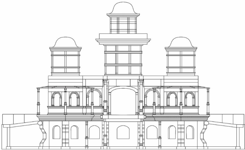
Figure 3. Frontal elevation of the Lingzhao Pavilion with indications of the Sumeru-base and the tri-part composition, rendered after a drawing in Fang Liyu, “The interdisciplinary research of virtual recovery and simulation of heritage buildings. Take Lingzhao Xuan in the Palace Museum as an example,” in
