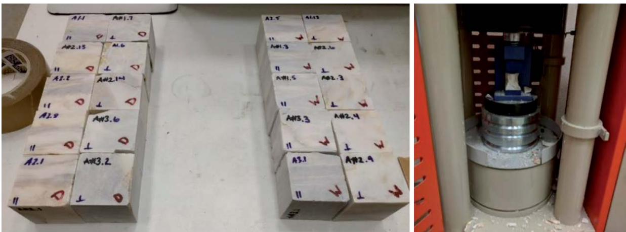
Figure 7: Northeast Temple, Antiochia ad Cragum. Left: prepared and labeled Antioch cube specimens (D=dry, W=wet, ||=parallel to grain, ⊥=perpendicular). Right: compression test of a marble specimen
