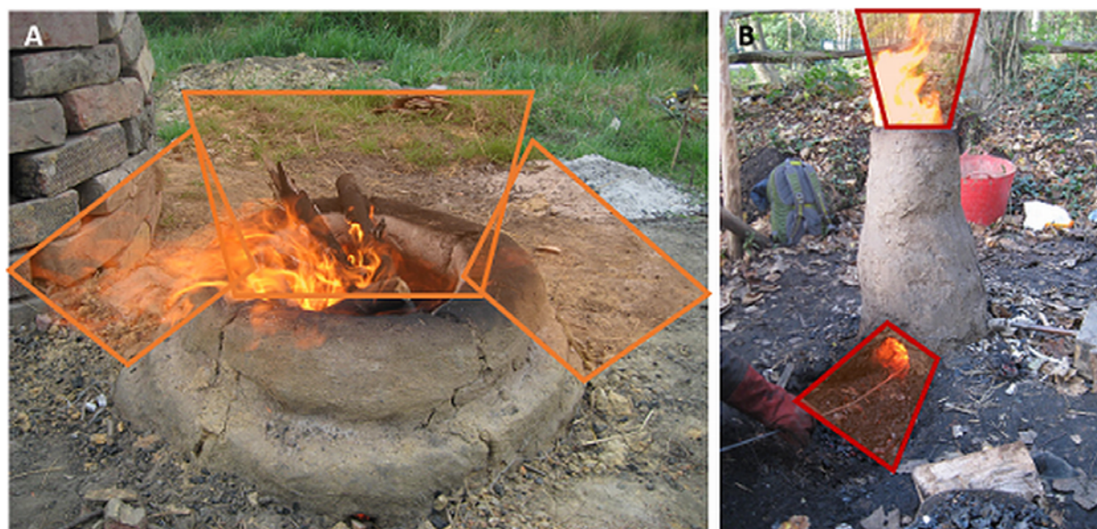
Figure 8: (A) The copper smelting furnace with shapes drawn to indicate the direction in which its heat radiates. (B) The iron smelting furnace with shapes drawn to indicate the direction in which its heat radiates.
