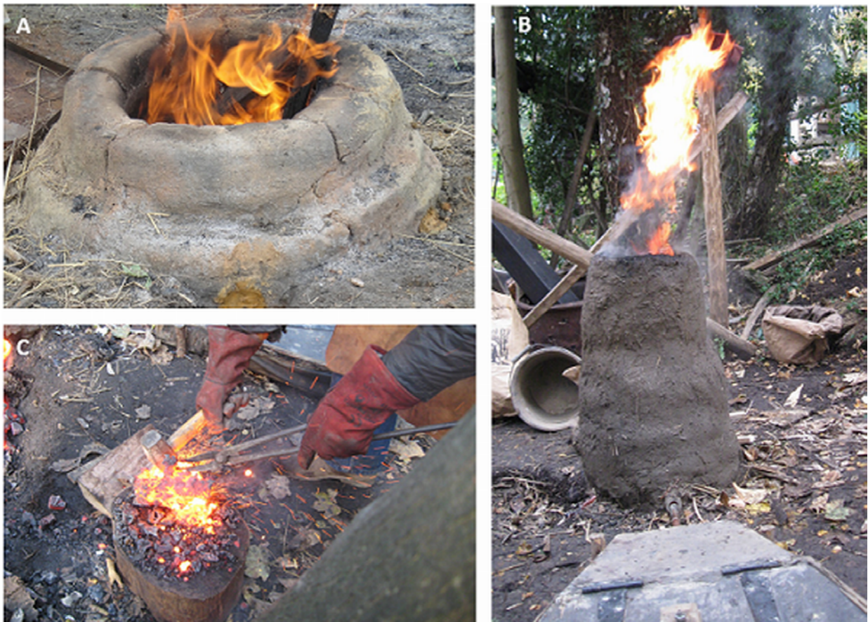
Figure 1: Examples of the variety of metallurgical practices undertaken. (A) Copper smelting furnace. (B) Shaft furnace for bloomery iron production. (C) Smithing of an iron bloom.
