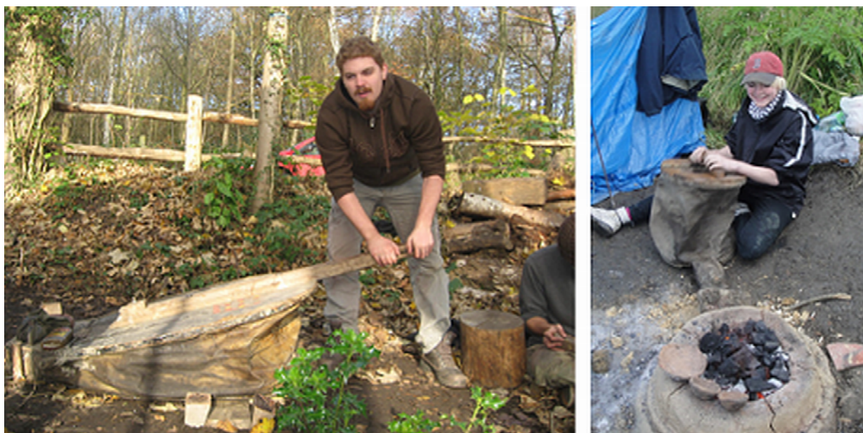
Figure 7: Images of bellows being used for forced draught with iron (left) and copper (right) smelting furnaces.
