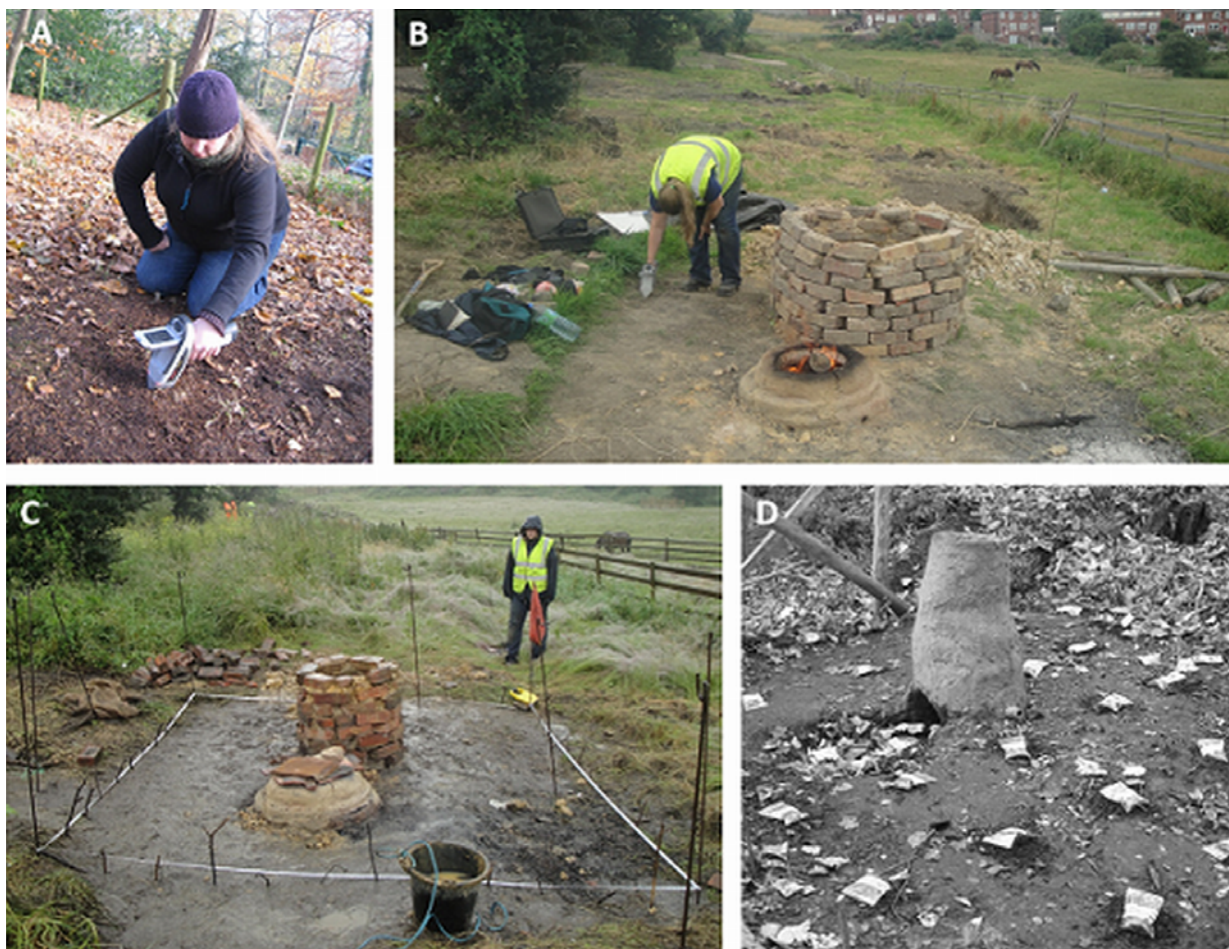
Figure 2: Various sites of experimental metallurgical activity. (A) The author using the pXRF in situ at a control site. (B) The copper smelting site being sampled in situ. (C) The copper smelting site showing the tape and stakes used to define the 0.25x0.25 m sampling resolution on the 3x3 m grid. (D) The iron smelting and smithing site where soil samples have been taken for ex situ pXRF measurement in the lab.
