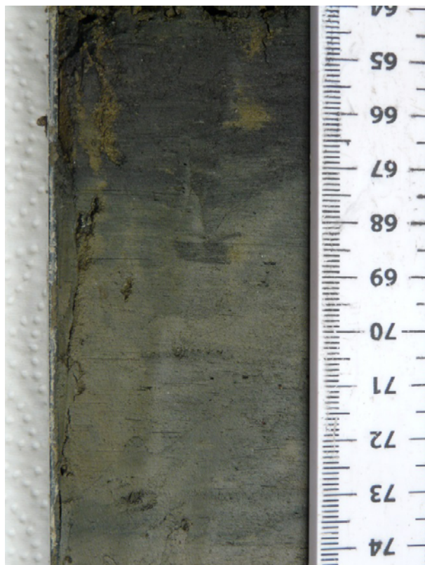
Figure 37. Photograph of the prepared surface of sediment sampled by a Russian corer at borehole 56a between 405.5 and 415.0 cm depth showing a transition from pale grey to black and bottle-green mud.
