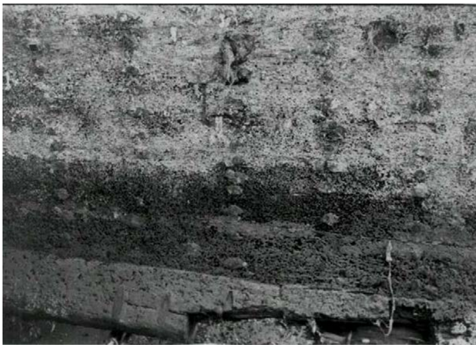
FIGURE 19: CLOSE-UP OF KEEL AND SIDE PLANKS OF ARAB DHOW SHOWING INTENSE INFESTATION OF MARINE WOOD-BORERS.
