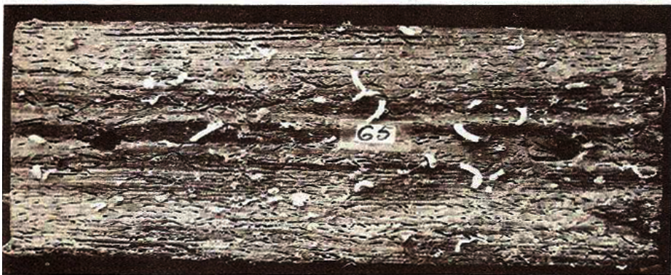
FIGURE 7 CALCAREOUS TUBES OF SHIPWORMS PROTRUDING FROM A PINE WOOD , LOOKING LIKE SERPULIDS. NOTE THE HEAVY INFESTATION OF LIMNORIA . (LOCALITY : TRONDHEIM, NORWAY).
