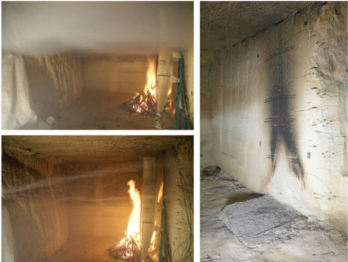
FIGURE 10. RELEASE AND DISSIPATION OF THE SMOKE (LEFT) AND SOOT DEPOSIT
