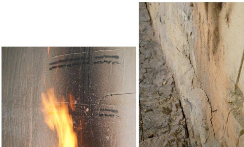
FIGURE 6. QUARRY OF LUGASSON. SOOT DEPOSIT AND SPALLING (LEFT) AND RUBIFICATION (RIGHT) (CREDITS C. FERRIER).
