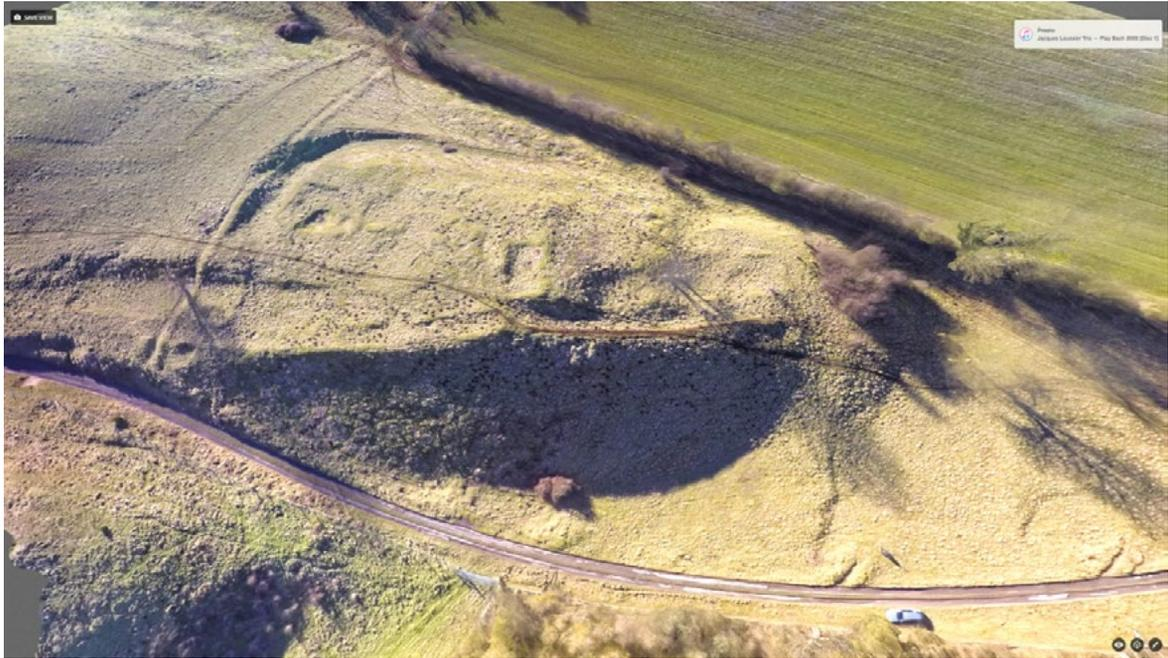
FIGURE 13. 3DI MODEL GENERATED FROM MORE THAN 150 IMAGES GATHERED USING A DJI QUADCOPTER WITH A GOPRO 4 CAMERA. REMARKABLY ISOLATED TREES ON THIS MONUMENT PHOTOGRAPHED IN FEBRUARY CAN BE SEEN FROM THEIR SHADOWS BUT WERE EXCLUDED FROM THE MODEL WITHOUT ANY HAND EDITING OWING TO THE NUMBER AND VIEW ANGLES OF THE COLLECTED IMAGES.
