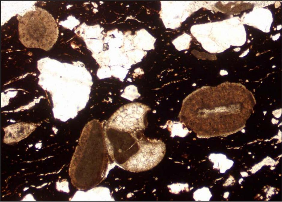
Fig. 1.19 An archaeological ceramic thin section seen at high magnification under the light microscope in plane polarised light (PPL). The dark brown is the clay matrix, which surrounds the white and light brown inclusions, as well as the white elongate voids. Compare with Fig. 1.20 below. Anglo-Saxon pottery, England. Image width = 2.9 mm.
