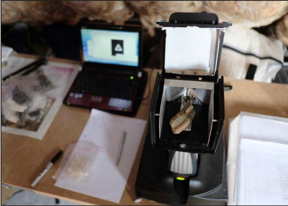
Fig. 1.17 Archaeological ceramic sherd being non-invasively geochemically characterised via portable X-ray fluorescence spectroscopy (pXRF). The sherd has been placed within a lead-lined chamber (open for illustrative purposes) over the beam and detector of the instrument, and data is being recorded on a laptop. Roman pottery, England.
