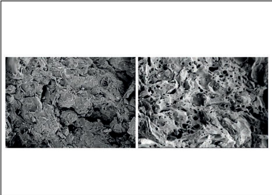
Fig. 1.15 Clay vitrification microstructure of archaeological ceramic sherds in the SEM. The sample on the left exhibits a rough appearance from the presence of the clay minerals, whereas on the right these have vitrified to form a glassy network. Neolithic pottery, Serbia. Image width = 0.1 mm (L) and 0.05 mm (R). Modified from Amicone et al. (2020, fig. 6).
