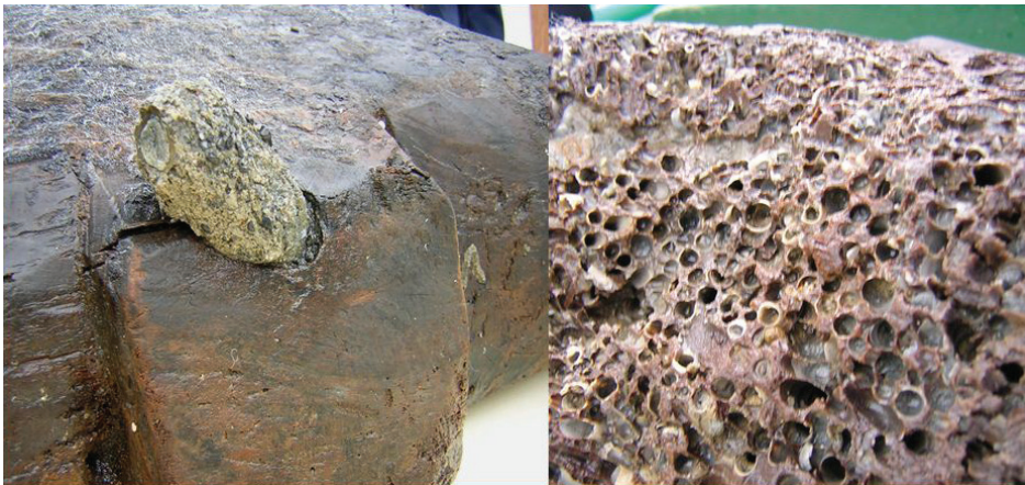
FIGURE 1: BORER-INFESTED ARCHAEOLOGICAL WOOD FRAGMENT, SHOWING EXTERNAL SOUND APPEARANCE (LEFT) AGAINST THE INTERNAL HONEY-COMBED STRUCTURE (RIGHT).
