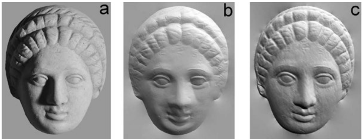
FIG. 7. SMALL CLAY ROMAN MASK: (A) ORIGINAL PHOTOGRAPH; (B) RECONSTRUCTED 3D MORPHOLOGY MAP WITH \alpha EQUAL TO 30^\circ ; (C) RECONSTRUCTED 3D MORPHOLOGY MAP WITH \alpha EQUAL TO 60^\circ .
