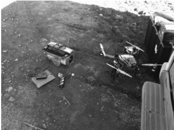
FIG. 2. THE CUSTOM MADE RPAS PLATFORM (DROIDWORX CX4) IN THE FIELD DURING THE BATTERY RECHARGING.
