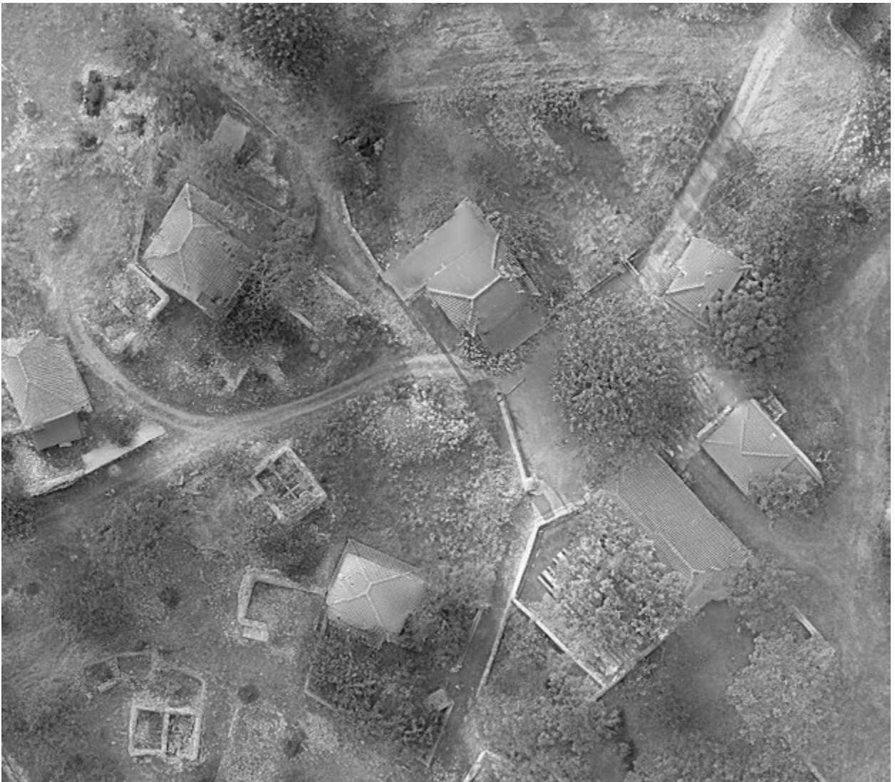
FIG. 8. SECTION FROM ORTHOPHOTO PRODUCED USING BARE EARTH SURFACE IN AGISOFT. NOTE THE 'GHOSTING' AROUND SEVERAL BUILDINGS WHERE THE SURFACE WAS INSUFFICIENT TO HOLD ALL FEATURES TO THE SAME SURFACE LOCATION.
