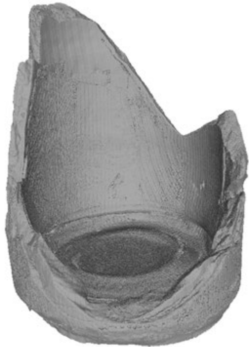
FIG. 7. EXAMPLE OF BASE FRAGMENT MODEL CREATED WITH DAVID SLS-1 STRUCTURED LIGHT SCANNER.
