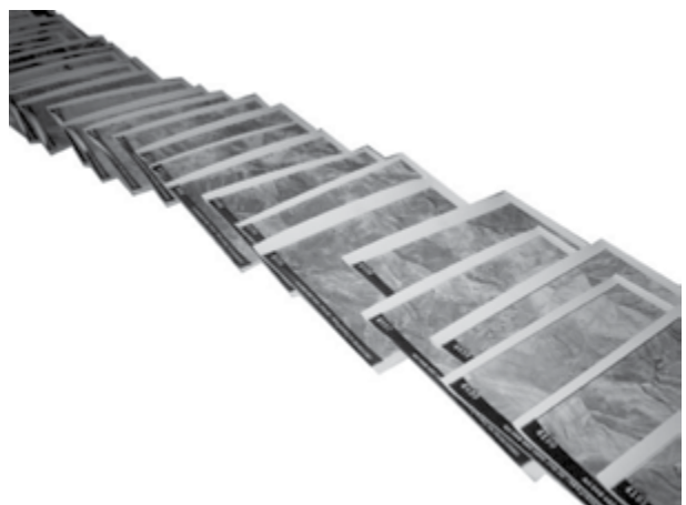
FIG. 1. AN ILLUSTRATION OF HOW PHOTOS WERE TAKEN DURING AN RAF FLIGHT OVER ITALY. THE INDIVIDUAL PHOTOS ARE PLACED IN THEIR CORRESPONDING POSITIONS. (© MIBAC-ICCD, AEROFOTOTECA NAZIONALE, FONDO RAF).
