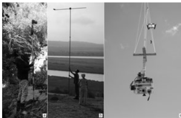
FIG. 2. CUSTOM-MADE DEVICES FOR 2D PHOTOGRAMMETRY (A, B) AND ALUMINIUM CRADLE FOR KITE (C).
