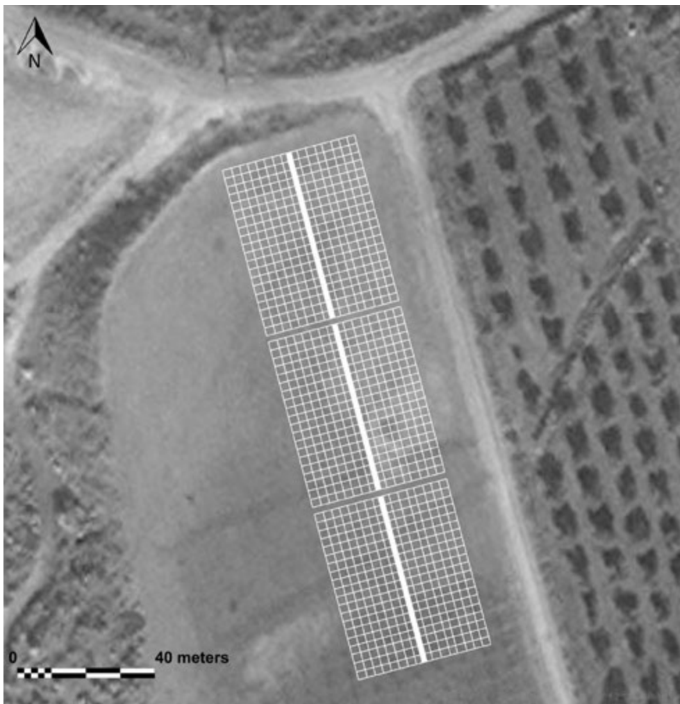
FIG. 6. EXAMPLE OF A CALIBRATION FIELD. THE TOTAL LENGTH OF THE GRID IS 150 M, DIVIDED INTO THREE 50 M SEGMENTS. THE WIDTH OF THE GRID IS 40 M (20 M ON EACH SIDE). THE GRID WAS ONLY MARKED BY TAPES DOWN THE CENTRE LINE.
