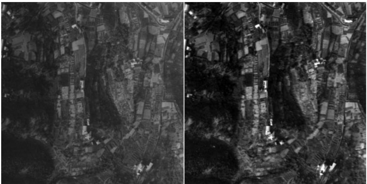
FIG. 9. BY LOOKING AT THE PHOTOGRAPH TO THE LEFT IT IS HARD TO TELL HOW THE LANDSCAPE IS SHAPED. THE ONLY CLUE TO THE DEPTH IS THE SHADOWS. THE ANAGLYPH STEREO IMAGE TO THE RIGHT, ON THE OTHER HAND, REVEALS THESE DETAILS CLEARLY.
