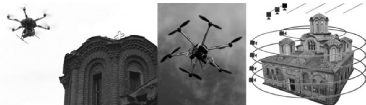
FIG. 3. UAV-BASED AERIAL DATA COLLECTION AND ILLUSTRATION VISUALIZATION OF THE MULTIPLE CLOSED LOOP PHOTO SHOOTING APPROACH.
