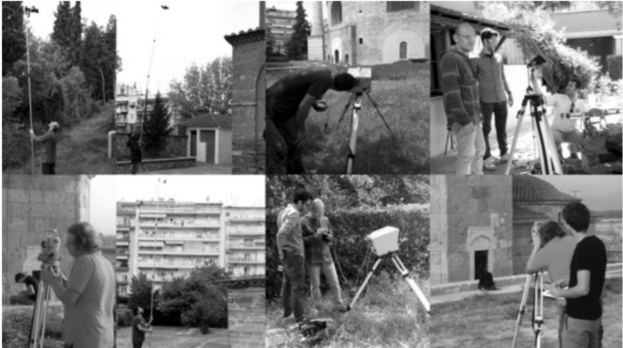
FIG. 2. TERRESTRIAL DATA COLLECTION USING DIGITAL CAMERAS, TIME-OF-FLIGHT LASER SCANNER, AND TOTAL STATION.
