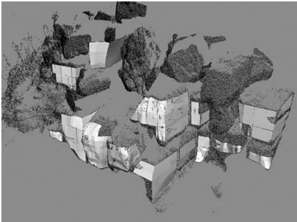
FIG. 7. POINT CLOUD PROCESSING OF THE ELEMENT E6.
