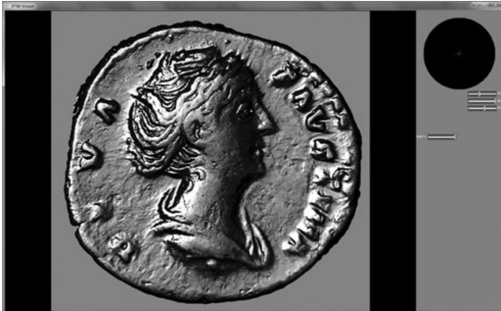
FIG. 1. VISUALIZATION OF OBVERSE OF COIN A THROUGH THE HEWLETT-PACKARD PTM VIEWER SOFTWARE, WITH VIRTUAL LIGHT SOURCE AT LEFT, IN SPECULAR ENHANCEMENT MODE. (LINDSAY MACDONALD 2015).
