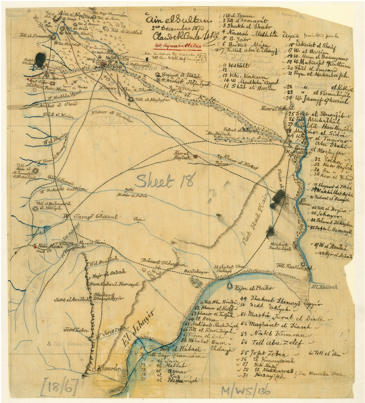
Figure 5. Original field tracing of the Jericho region from the Survey of Western Palestine. Drawn by Claude Conder on 2 December 1873. Courtesy of the PEF archives (PEF-M-WS-136).
