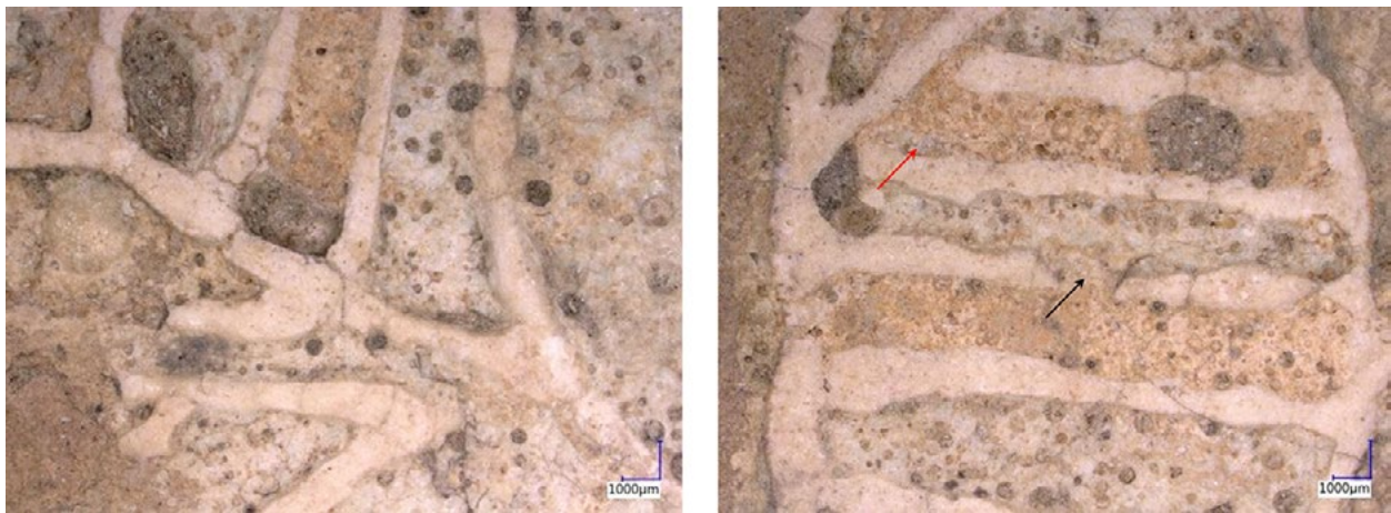
Figure 7. Micro-photographs of ME 92183 showing details of the white paste applied on top of the coloured glazes as an outline for the figures. Note a) the different thickness of the lines and the overlap in some areas (20x) and b) the presence of coloured glass in the areas where the white outline is lost (indicated with arrows), informing about the manufacturing sequence (Lucia Pereira-Pardo).
