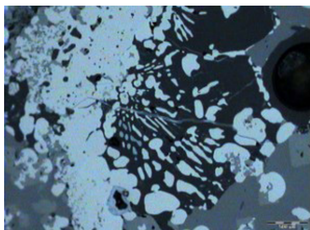
Figure 14. Photomicrograph of iron slag showing the presence of metallic iron (Fe; lighter areas), wustite (Wus; light grey patches in dark grey), fayalite (Fay; dark grey) and silicate as matrix. Scale bar is 500 \mu\text{m} . From Naizatul Akma Mokhtar and Mokhtar Saidin (2018b: photo 3).
