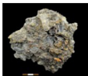
Figure 7. Iron slag, amorphous with a base. From Naizatul Akma Mokhtar and Mokhtar Saidin (2018a: photo 8).
