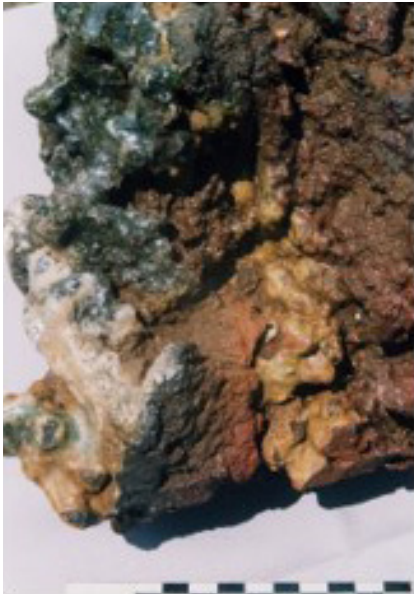
Figure 10. Internal layering of Furnace #1 wall. Photo: D. Hein.
