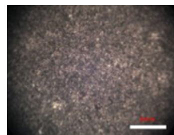
Figure 11. Fine mineral in cherty metasediment. White bar is 1 mm long. Photo: Nor Khairunnisa Talib (2013).
