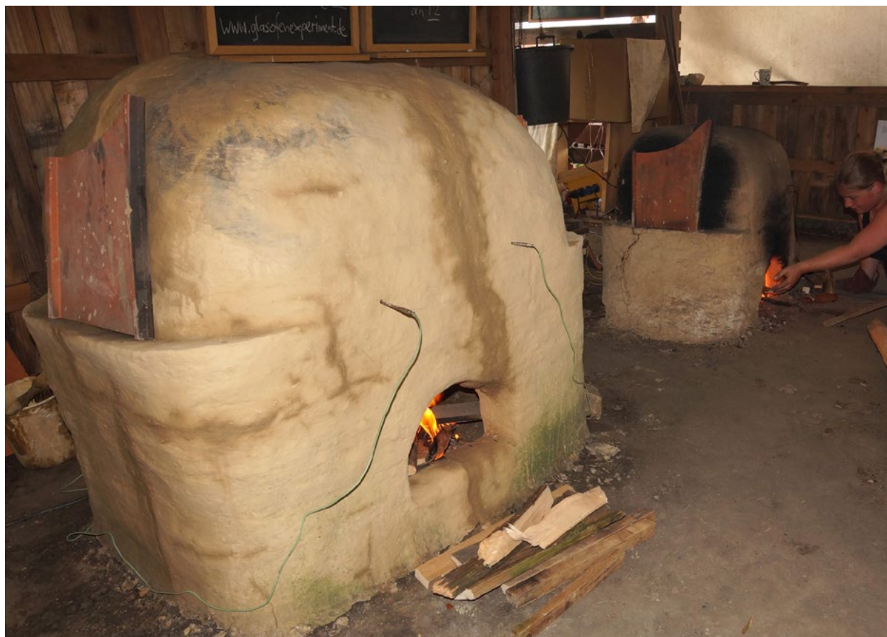
Figure 9: Large and small annealing ovens KO-Borg-2 and KO-Borg-1 (Photo: Frank Wiesenberger).
