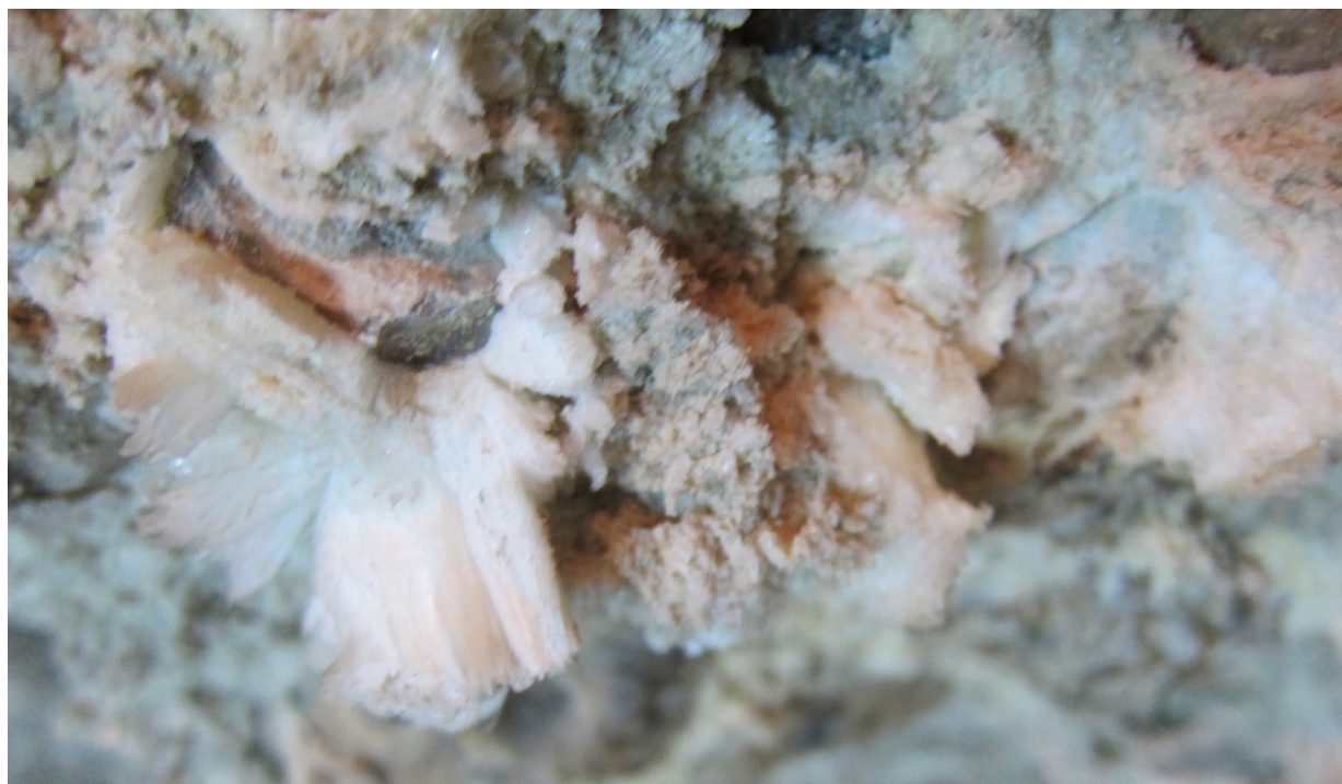
Figure 5. Salt crystallization in a non-royal saff tomb (photo R. Soliman, February 2017).
