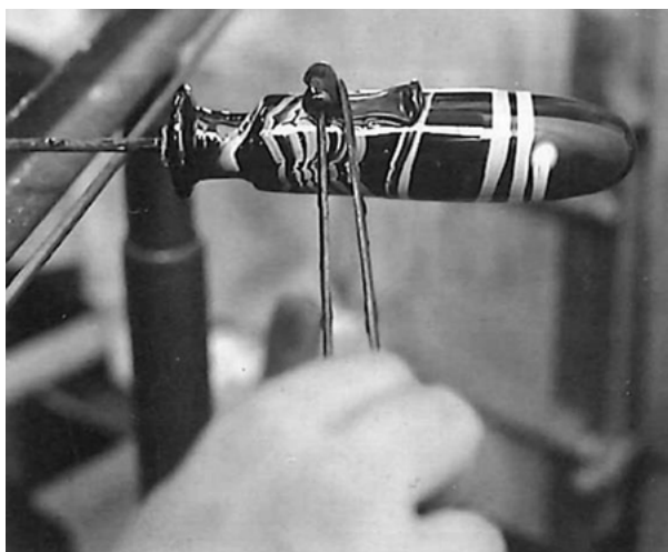
Figure 4.51: Forming 'duck-head' handles using pincers (Tait 1991: 215, fig. 13).
