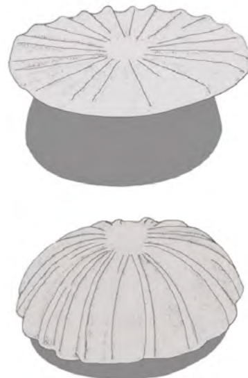
Figure 4.13: The principle of slumping a glass blank – here with ribs – over a dome-shaped mould. The heat in the kiln causes the glass disc to slump down over the form (after Grose 1989: 245, fig. 118).
