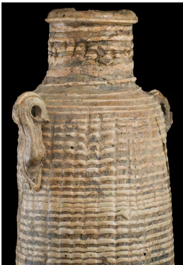
Figure 4.61: Vertical depressions on the surface of a core-formed glass vessels creating a fluted body. The depressions are due to insufficient smoothing of the surface during the finishing process (courtesy of The Corning Museum of Glass).
