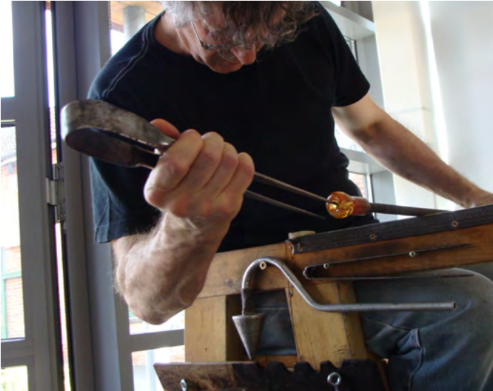
Figure 4.38: Next, a central hole is made by inserting a sharp tool into the gather, which will later become the central hole of the rosette (published with the permission of the 'Roman Glassmakers'). The glass is allowed to cool and stiffen before gathering a second layer of melted glass over it.
