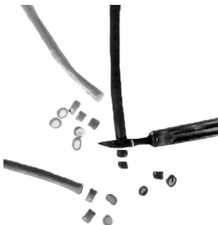
Figure 4.1: Cutting of mosaic rods, carried out in cold state while it is still plastic (after Wartke 2012: 409, fig. 5).
