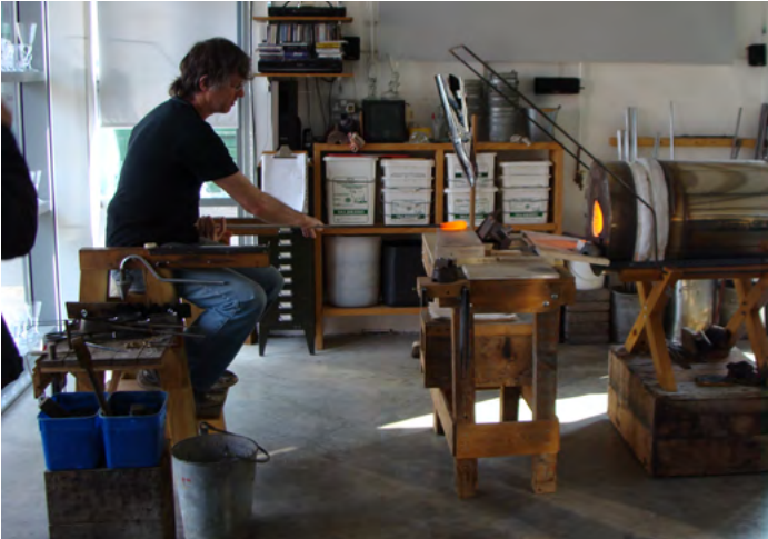
Figure 4.37: Viscous glass is gathered* on an iron and marvered* on a stone surface (published with the permission of the 'Roman Glassmakers').
