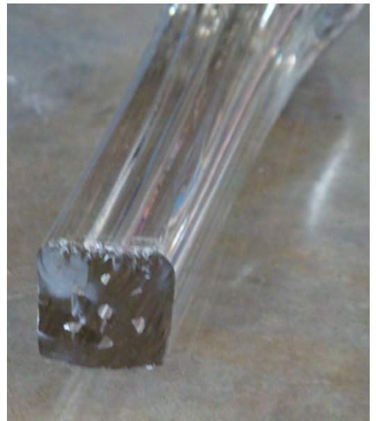
Figures 4.42, 4.43: A rod of the desired thickness is formed by reheating and stretching the glass (published with the permission of the 'Roman Glassmakers').
