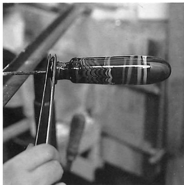
Figure 4.50: Forming the neck using pincers (Tait 1991: 215, fig. 10).
