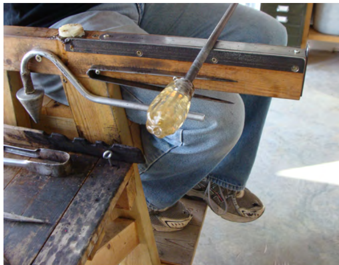
Figures 4.39, 4.40, 4.41: Using a pair of pincers, six slots are created in the hot glass. These slots will form the petals of the rosettes. The glass is allowed to cool and harden (whilst slowly turning the iron) (published with the permission of the 'Roman Glassmakers'). A third layer of hot glass is added, trapping air in the slots and creating hollow spaces. Using the marver, the glass is carefully shaped to achieve a square cross-section.
