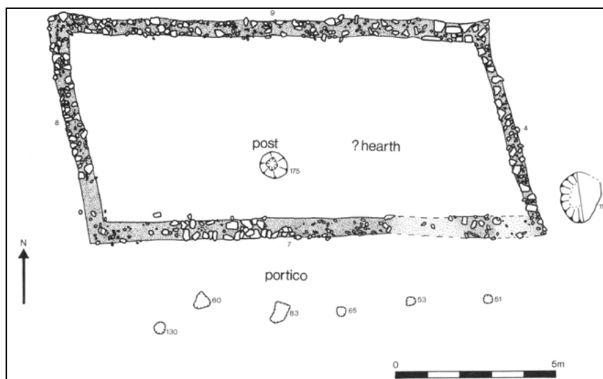
FIGURE 5.24. PLAN OF FARMHOUSE AT PODERE TARTUCHINO, PHASE I (PERKINS AND ATTOLINI 1992: 80). NOTE THE CENTRAL POST HOLE, WHICH LIKELY HELD THE RIDGE POLE.
