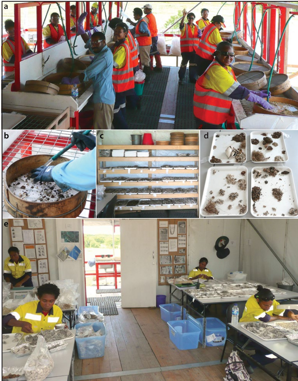
FIGURE 9.6. WET SIEVING AND SORTING OPERATIONS IN THE CAUTION BAY FIELD LABORATORY, SEPTEMBER 2009 – MAY 2010 (PHOTOS: CASSANDRA ROWE): A. WET SIEVING TEAM AT WORK; B. CLOSE-UP OF WET SIEVING THROUGH 2.1MM MESH SIEVE; C. WET SIEVE RESIDUE ON TRAYS DRYING ON SHELVES PRIOR TO SORTING; D. SORTED SIEVE RESIDUE ON TRAYS; E. SORTING TEAM AT WORK ON SIEVE RESIDUE.
