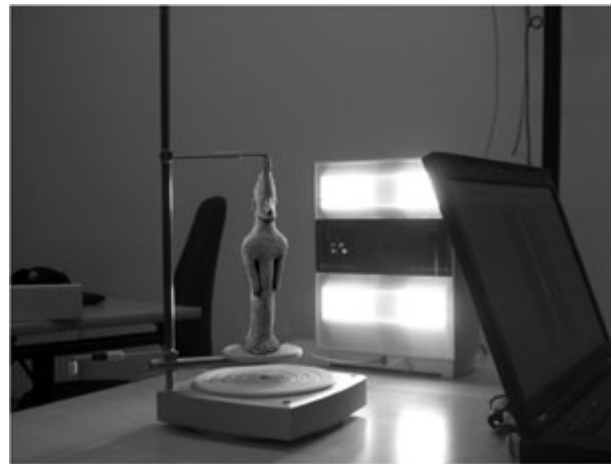
FIG. 3. DATA ACQUISITION OF A TERRACOTTA WITH NEXTENGINE 3D DESKTOP LASER SCANNER.
