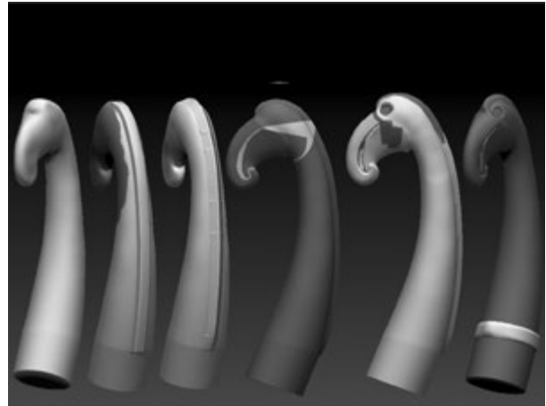
FIG. 4. SCREEN SHOT SHOWING STAGES OF THE DIGITAL CARVING PROCESS IN THE COMPUTER PROGRAM Z-BRUSH.
