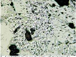
5 – fused lattice structures of wüstite with the border of a primary grain (white), polygonal and prismatic crystals of fayalite (grey).
