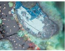
2 – Pokrovskoe, sample 1313, 4th mineralogical group, length of the photo is 0.62 mm, crossed nicols: large grain of covellite (blue) included into the malachite grain (light green); small copper prills nearby in the glass matrix.
