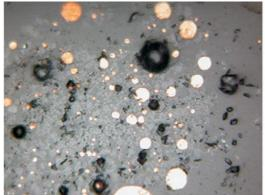
1 – sample 2025, Baytu – Accumulation of magnetite particles disintegrating from a larger grain. Copper prills are inside.
