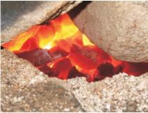
1 – Smelting of oxidized ores is carried out almost without smoke and flame. Color of the charcoal makes possible to distinguish areas with different temperatures. Thus, under the upper layer of charcoal there is an area of thermal maximum.
