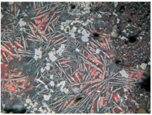
1 – Microstructure of slag of experimental smelting 5. Length of the photo is 0.54 mm. Delafossite needles, dendrites of cuprite (cherry-colored) and octahedral of magnetite in glass matrix.
