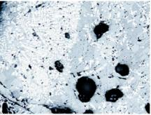
2 – fused dendrites of wüstite (white) and molten disintegrating grain of wüstite formed from another iron oxide (on the left), polygonal and needle-shaped crystals of fayalite (light grey) in glass (dark grey matrix) with small pores (black).
