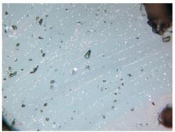
6 – Tokskoye, sample 1292, 4th mineralogical group, length of the photo is 0.62 mm: small prills of copper forming in some instances long curved chains.
