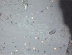
4 – sample 2024 – Copper prills and accumulation of fine dendritic skeletons of magnetite in the glass matrix.
