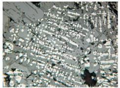
3 – Skorodum, sample 149 (length of the photo is 0.54 mm), prismatic crystals of olivine and lattice structures of wüstite.
