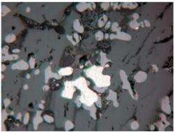
6 – small grains of chalcopyrite (white), prismatic crystals of fayalite (grey) and remains of fused dendrites of wüstite (light grey).
