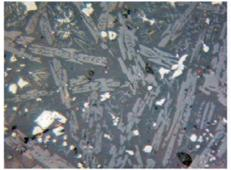
Palatki I, sample 139 (length of the photo is 0.22 mm), long skeletal prisms of olivine (light grey), small octahedra and particles of magnetite (white), pores (black), copper prills.
