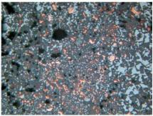
6 – Microstructure of slag of experimental smelting 5. Length of the photo is 0.54 mm. Accumulations of copper particles among the particles of iron oxide in glass matrix.
