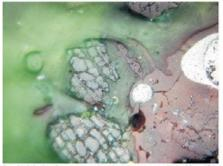
3 – A globule of copper and malachite surrounded with sulfide border in the painted glass matrix. A fused grain of malachite and quartz particles forming a structure of sandstone (length of the photo is 0.62 mm, crossed nicols).
