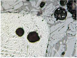
3 – prismatic crystals of fayalite (grey), accumulation of fused lattice structures of wüstite with the border of a primary grain (white) and pores (black) in the glass matrix (dark grey).
