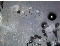
2 – Typical microstructure of ceramic slag. Sample 2155, experimental smelting 8, length of the photo is 0.54 mm. Light gray needles of fayalite crystallization and pores (dark) in the dark grey glass matrix.
