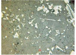
3 – Itkul I, sample 109 (length of the photo is 0.54 mm), badly visible small prisms of olivine (grey), skeletons, small dendrites and octahedra of magnetite (white) and copper prills.
