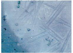
5 – sample 2353, slagged lining: needleshaped crystals of fayalite and copper prills.
