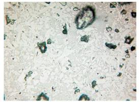
3 - sample 574, Besh-Bulak 4, accum. 2: middle part of slagged ceramic crust (glass with small prisms of olivine).
