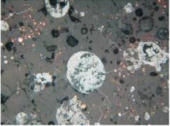
5 – sample 2023 – Large globule of sulfide with copper inclusions and cuprite border, prills of cuprite and copper, small cracks filled with cuprite, pores (length of the photo is 0.62 mm).
