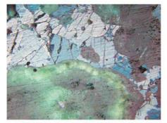
5 – Ivanovskoye, sample 1304, 2nd mineralogical group, length of the photo is 0.62 mm: ore grain consisting of malachite (green) and covellite (blue).
