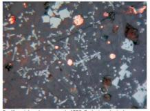
5 – Kuzminkovskoye, sample 1285, 2nd mineralogical group, length of the photo is 0.54 mm: small octahedral, skeletons and dendrites of magnetite, copper prilis; crystallizing silicates (probably, olivine) are slightly distinguishable against the background of the glass matrix.
