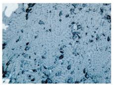
6 – dense small skeletal crystals of fayalite (grey) in the dark grey glass, fused grain of wüstite (light grey).
