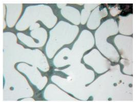
6 – Partizanskaya Katushka, sample 781, fused grains of wüstite (length of the photo is 0.22 mm).
