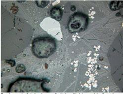
3 – long skeletal prisms of olivine (light grey) in the glass matrix (grey), grains of quartz (dark grey), a grain of chromite (grey with a white magnetite border), octahedra of magnetite (white) and pores (length of the photo is 0.22 mm).
