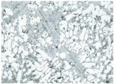
5 – fused grains of wüstite (white) against the background of long prismatic and needle-shaped crystals of fayalite (grey) in the glass matrix (dark grey).
