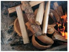
3 - The firing of tuyeres and crucibles in the open fire,
