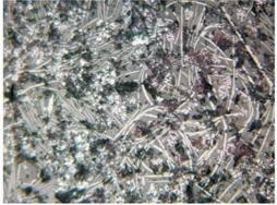
5 – sample 2026 – Thin curved needles of delafossite, dendrites and prills of cuprite, iron hydroxides.
