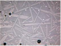
3 – Microstructure of slag of experimental smelting 10. Length of the photo is 0.54 mm. Prisms and needles of olivine and small rash of magnetite.
