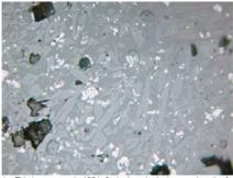
1 – Tokskoye, sample 1291, 2nd mineralogical group, length of the photo is 0.62 mm: small long prisms of olivine (light grey) in the glass matrix (dark grey), small particles of magnetite and wüstle (light) and very small copper prills.
