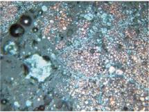
4 – Kuzminkovskoye, sample 1280, 4th mineralogical group, I ength of the photo is 0.62 mm: Accumulation of copper prils, prills and grains of cuprite (blue). Cuprite fills also cracks in the glass matrix.
