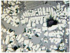
5 – Turbino I, sample 317 (length of the photo is 0.22 mm), polygonal crystals of olivine (light grey) in the glass matrix (dark grey) and fused large dendrites of wüstite (white).
