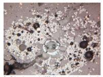
5 – Pokrovskoe, sample 1325, 4th mineralogical group, length of the photo is 0.62 mm: Round grain of chrysocolla in covellite border and copper prills in the accumulation of magnetite partic les disintegrating from a larger grain.
