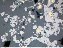
5 – Microstructure of slagged lining, sample 2165. Length of the photo is 0.54 mm. Grain of iron oxide disintegrating into particles and copper inclusions.
