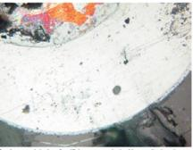
2 – Large globule of sulfide surrounded with cuprite border. There is a copper core inside, separated from the sulfide by a rim of cuprite (length of the photo is 0.62 mm).
