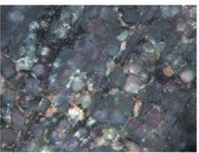
2 – Tokskoye, sample 1291, 2nd mineralogical group, length of the photo is 0.62 mm: sandstone with thin malachite 'cement'.
