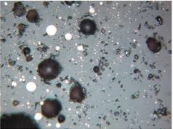
6 – sample 1846 – Copper prills and pores in the glass matrix.
