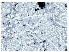
6 – Biktimirovo settlement, sample 2349: fused dendrites of wüstito (white) against the background of prismatic crystals of fayalite (light grey) in the glass (dark grey matrix) with small pores (black).
