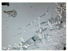
6 – sample 518, 6th mineralogical group, 3rd type, Lyavlyakani 26: large polygonal and smaller prismatic crystals of olivine (dark grey) formed after crystallization of dendrites of wüstite (white), small pores (black).
