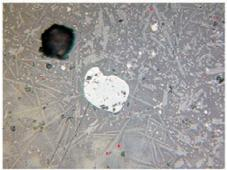
3 – Palatki I, sample 140 (length of the photo is 0.54 mm), needles and small prisms of olivine (light grey), chromite grain (in the center), small magnetite crystals and copper prills.
