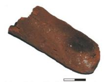
$4-\mbox{Tuyere}$  after its use. It is well visible that the tuyere is slagged.
