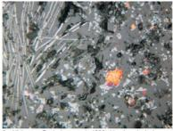
2 – Nizhnyaya Pavlovka, sample 1286, 4th mineralogical group length of the photo is 0.46 mm: octahedral and skeletons of magnetite (light), copper prils and needles of delafossite. Some prils of copper are shapeless, magnetite forms around them.
