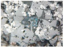
5 – Polygonal crystals of olivine (grey), and magnetite octahedral (white) formed earlier. A blue grain of covellite in the center (length of the photo is 0.46 mm).
