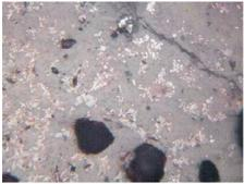
1 – sample 2032, 4th mineralogical group, 3rd type, Kelleli 4: small octahedra of magnetite (grey), prills of copper and dendrites of cuprite (red fields with white inclusions).
