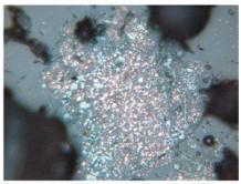
4 – Tokskoye, sample 1293, 4th mineralogical group, length off the photo is 0.46 mm: accumulation of mol-ten inclusions of copper and cuprite keeping the form of a primary ore grain.
