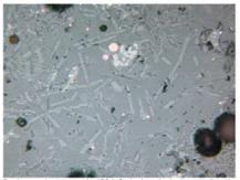
3 – Ivanovskoye, sample 1304, 2nd mineralogical group, length of the photo is 0.62 mm: large needle-shaped skeletons of olivine in the glass matrix, rare copper prills and pores (black).
