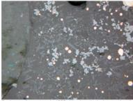
3 – Ivanovskoye, sample 1305, 4th mineralogical group, length of the photo is 0.48 mm: particles, skeletons and dendrites of magnetite (tight), copper proliis in the glass matrix; a large grain of malachite with small inclusions of covellite (blue) on the left. Some copper prills (in the upper right corner) have a thin sulfide border.
