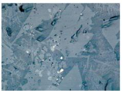
6 – sample 2354, slagged lining: polygonal crystals of fayalite, its small needle-shaped crystals, copper prills, small octahedra of magnetite (light grey).
