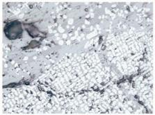
3 – lattice structure of fused dendrites of wūstite (white) saved border of a primary ore grain, long prismatic and needle-shaped crystals of fayalite (light grey) in the dark grey glass with pores (black).
