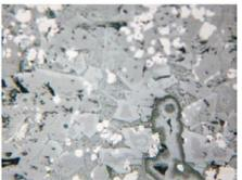
6 – Small dendritic skeletons and crystals of magnetite, olivine crystals with zonal structure: the outer part is lighter (length of the photo is 0.46 mm).
