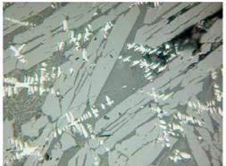
3 – crystallizing from the slag fused dendrites of wüstite (white) and prismatic crystals of fayalite (grey).
