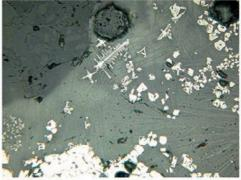
6 – Turbino I, sample 318 (length of the photo is 0.22 mm), long skeletal prisms of olivine (greenish-grey), dendrites, skeletons and particles of magnetite (white), grain of quartz (dark grey).
