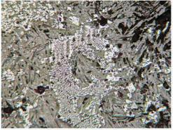
5 – Itkul I, sample 114 (length of the photo is 1.55 mm), needle-shaped and small prismatic crystals of olivine (grey), octahedra of magnetite and lattice fused structure of magnetite saved the border of a primary grain.
