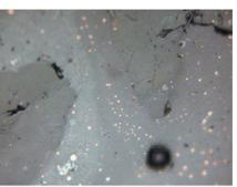
2 – Rodnikovskoye, sample 1332, 4th mineralogical group, length of the photo is 0.62 mm: quartz grains with fused borders and prills of copper, small skeletons of magnetite.
