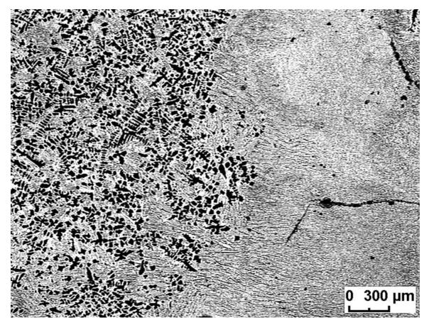
FIG. 13-1. CARBURIZED INCLUSIONS IN IRON (SAMPLE 66) FROM THE SETTLEMENT OF VERKHNYAYA ALABUGA.
