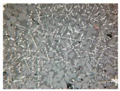
6 – 528, 3rd mineralogical group, 4th type, Ayakagitma 209: dendrites of magnetite, small prisms of olivine and prills of copper.
