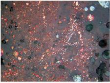
5 – Palatki I, sample 141 (length of the photo is 0.54 mm), small copper prills and larger globules of cuprite (light blue), fused particles of malachite (greenish).
