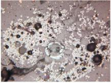
3 – Pokrovskoe, sample 1325, 4th mineralogical group, length of the photo is 0.62 mm: accumulation of magnetite particles disintegrating from a larger grain, round grain of chrysocolla within the border of covellite and copper prills.
