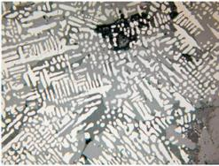
Large lattice structures of fused dendrites of wüstite (white), joint polygonal crystals of fayalite (grey).
