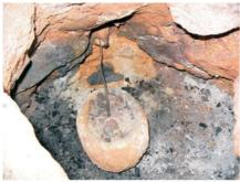
1 – Furnace and smelting bowl after operation. The stick shows the direction of blowing from the tuyere. The red color around the tuyere demonstrates the area of the oxidizing conditions. The black walls show the area of the generation of carbon dioxide. The upper part of walls is red due to coming of air from above.
