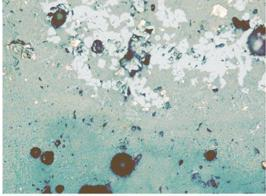
3 – sample 2455, copper prills, magnetite particles separating from a larger grain and small dendrites of magnetite.
