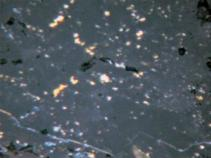
4 – Microstructure of slagged lining, sample 2165. Length of the photo is 0.22 mm. Copper prills in the glass matrix.
