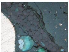
5 –Pokrovskoe, sample 1312, 4th mineralogical group, length of the photo is 0.62 mm, crossed nicols: fragment of sandstone (diagonal strip through the photo), malachite; large globule of copper on the left, small needles of delafossite and small copper prills on the right.
