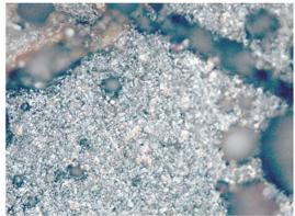
1 – sample 2479, copper prills in the slagged ceramic mass.
