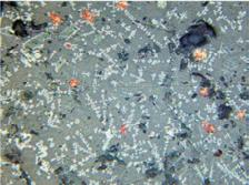
4 – Palatki I, sample 141 (length of the photo is 0.54 mm), skeletons of magnetite and copper prills, particles of malachite (green).
