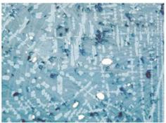
4 – sample 2431, slag: needle-shaped crystals of fayalite (background), dendrites of magnetite and copper prills.
