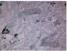
2 – sample 544, 2nd mineralogical group, 1st type, Besh-Bulak 3: long prismatic crystals of olivine (dark grey) in the light glass matrix, particles of magnetite (white) and copper prills.
