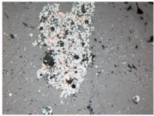
1 – Ivanovskoye, sample 1307, 2nd mineralogical group, length of the photo is 0.62 mm: accumulation of fused particles of magnetite, which keeps borders of a primary ore grain. It contains inclusions of copper sulfide (blue ones in the upper part of the 'grain') and small copper prills.
