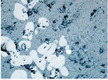
4 – fused dendrites of wüstite (light grey) in glass (dark grey, matrix) filled with dense small skeletal crystals of fayalite (grey), fused particle of iron (white).
