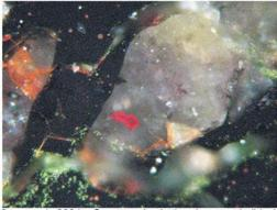
3 – sample 2024 – Quartz grains in the glass matrix (black). Cuprite inclusion (red) in quartz.
