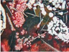
4 – Pokrovskoe, sample 1319, 4th mineralogical group, length of the photo is 0.46 mm, crossed nicols: dendrites and molten inclusions of cuprite and needles of delafossite.
