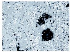
fused dendrites of wüstite (white) against the background of prismatic crystals of fayalite (light grey) in glass (dark grey matrix) with small pores (black).
