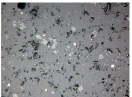
2- sample 2025, Baytu – Octahedra of magnetite, copper prills and pores in the glass matrix.
