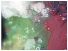
1 – Grains of quartz, malachite and chrysocolla in the glass in the red color by small particles of cuprite (length of the photo is 0.62 mm, crossed nicols).
