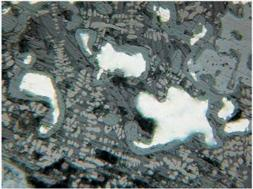
4 - Irtyash II, sample 2214, fused dendrites of wüstite and inclusions of iron surrounded with hydroxides.
