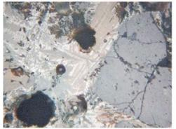
3 – sample 2023 – Quartz grains, dendrites of hydroxides and pores (length of the photo is 0.62 mm).
