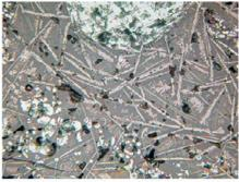
1 – Pokrovskoe, sample 1311, 4th mineralogical group, length of the photo is 0.54 mm: large grain of malachite (light green), prills of cuprite (light) and needles of dela-fossite, on edges of the latter and around the dendrites of cuprite grow.
