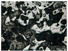
5 – sample 511, 6th mineralogical group, 3rd type, Lyavlyakan, 26: porous lower part of slagged ceramic crust.
