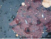
5 – Pokrovskoe, sample 1323, 4th mineralogical group, length of the photo is 0.62 mm: accumulation of molten inclusions of copper and cuprite keeping the form of a primary ore grain, long inclusions of unmolten sulfide (blue) in the center of the grain.
