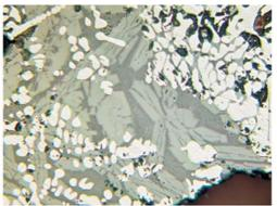
2 – Upper zone of the slag. Fused inclusions of wüstite (white), some particles are grouped and keep borders of a primary grain. Skeletal prisms of fayalite (grey).
