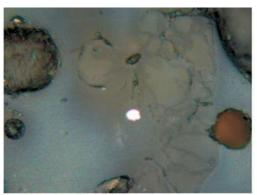
2 – fused grain of quartz and a copper prill in the porous glass (length of the photo is 0.22 mm).
