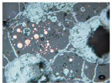
5 – Rodnikovskoye, sample 1331, 4th mineralogical group, length of the photo is 0.62 mm: accumulation of copper prills and large globules of cuprite (blue) that fills cracks.
