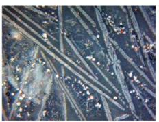
2 – Palatki I, sample 140 (length of the photo is 0.22 mm), long needles of olivine, small octahedra of magnetite and small copper prills.
