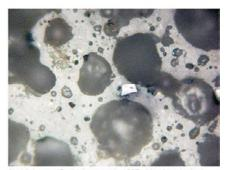
6 – Nizhnyaya Pavlovka, sample 1287, 4th mineralogical group, length of the photo is 0.62 mm: ceramic slag of the lining – very porous glass matrix with very small nuclei of olivine crystallization, small grains of quartz, rare small chromites.
