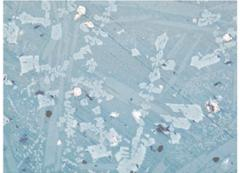
3 – sample 2431, slag: long prismatic crystals of fayalite, dendrites and skeletons of magnetite, copper prills.
