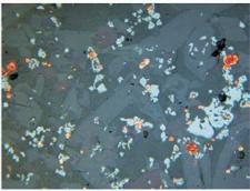
6 – Palatki I, sample 143 (length of the photo is 0.54 mm), prismatic crystals of olivine (grey), octahedra of magnetite and copper prills.
