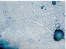
2 – crystals of delafossite (long needles) and small octahedra of magnetite (lighter crystals).
