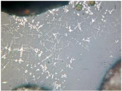
1 – Ostrovnoe III, sample 790 (length of the photo is 1.55 mm), small dendrites of magnetite.
