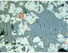
1 – Palatki I, sample 145 (length of the photo is 0.54 mm), long needles of olivine, large octahedra of magnetite and coppor prills.
