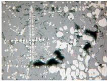
Uzhovoy Island, sample 2212, dense polygonal crystals of fayalite (light grey background), dendrites and fused grains of wüstite (white).
