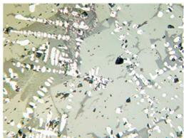
6 – fused dendrites of wüstite and polygonal crystals of fayalite.
