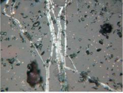
1 – sample 1846 – Pores, cuprite in the cracks and small copper prills in the glass matrix (length of the photo is 0.46 mm).
