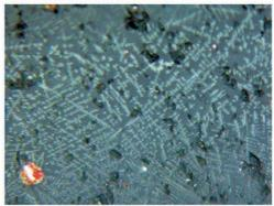
4 – Itkul I, sample 111 (length of the photo is 0.54 mm), smal dendrites of magnetite and copper prills in the glass matrix.
