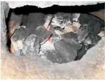
1 - Large pieces of birch charcoal allow air to circulate freely in the furnace.
