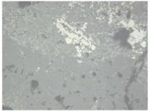
3 – Microstructure of slagged lining, sample 2165. Length of the photo is 0.54 mm. Light grey prisms of olivine, lighter particles of magnetite and small pink copper prills in the silicate glass matrix (grey background).
