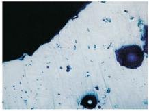
3 - Ulak-6, sample 2338. Small nuclei of fayalite crystallization in the porous glass.
