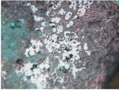
3 – Pokrovskoe, sample 1312, 4th mineralogical group, length of the photo is 0.62 mm, crossed nicols: disintegrating malachite grains (greenish), prills of cuprite and needles of delafossite.
