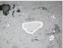
2 – Tokskoye, sample 1291, 2nd mineralogical group, length of the photo is 0.62 mm: small prisms of olivine (light grey) in the glass matrix (dark grey), small particles of magnetite and wüstite (light), in the center – chromite grain in the magnetite border, black porces.
