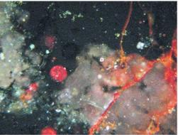
2 – sample 2024 – small prills of copper and larger globules of cuprite in the glass matrix. Cracks in the glass and quartz are filled with cuprite.
