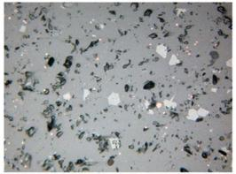
$3-\mathsf{sample}$  2025, <code>Baytu</code> – Octahedra of magnetite, prills and pores in the glass matrix. One copper prill is included into magnetite.
