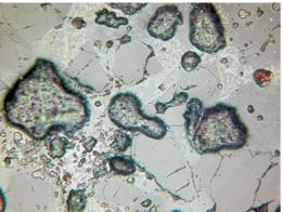
2 – sample 574, 6th mineralogical group, 3rd type, Besh-Bulak 4, accum. 2: lower part of slagged ceramic crust (quartz and ceramic mass, glass, small prisms of olivine).
