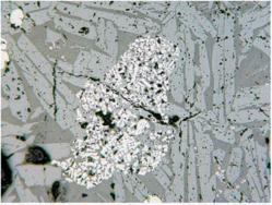
4 – fused lattice structure of wüstite with borders of a primary grain, long prismatic crystals of olivine (light grey) (length of the photo is 0.54 mm).
