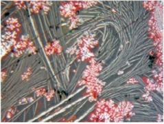
5, 6 - Pokrovskoe, sample 1311, 4th mineralogical group, length of the photo is 0.46 mm, crossed nicols: dendrites of cuprite and needles of delafossite.
