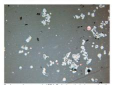
6 – Ivanovskoye, sample 1304, 2nd mineralogical group, length of the photo is 0.62 mm: large skeletons of magnetite and copper prills.
