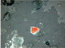
3 – sample 584, 4th mineralogical group, 3 type, Besh-Bulak 1, area 8: grain of copper surrounded with cuprite in the melting quartz grain (dark grey), in the upper right corner – small copper prills in the glass matrix.
