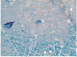
4 – sample 2455: copper prills, dendrites of magnetite and needles of delafossite in the glass painted with cuprite.
