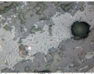
Ivanovskoye, sample 1305, 4th mineralogical group, length of the photo is 0.46 mm: small needles of delafossite, copper and malachite among the fragments of sandstone.
