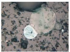
4 – Tokskoye, sample 1291, 2nd mineralogical group, length of the photo is 0.46 mm: large roundish grains of malachite (grey with greenish tint) with an adjoining to them molten prill of covellite (blue) in the glass matrix (dark grey), a large pore in the upper part.
