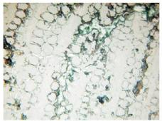
3 - Ivanovskoye, sample 1307, 2nd mineralogical group, length of the photo is 0.62 mm: sandstone with inclusions of malachite.
