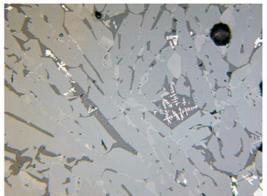
sample 518, Lyavlyakan, 26a: large long prismatic crystals of olivine and small dendrites of wüstite in the glass matrix.
