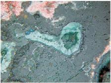
4 – sample 584, 4th mineralogical group, 3rd type, Besh-Bulak 1, area 8: malachite and cuprite in the quartz rock.
