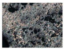
6 – Microstructure of gangue (sample 2156) of experimental smelting 8. Length of the photo is 1.55mm. Reduced particles of copper in the gangue.
