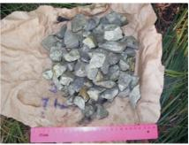
2 - Pieces of chalcopyrite (3-4cm) prepared for smelting.
