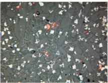
2 – Microstructure of slag of experimental smelting 5. Length of the photo is 0.54 mm. Prisms of olivine, skeletons and dendrites of magnetite, particles and prills of copper.
