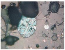
4 – Prills of covellite (blue), cuprite (white), small prills of copper and pores in the painted glass matrix (length of the photo is 0.46 mm).
