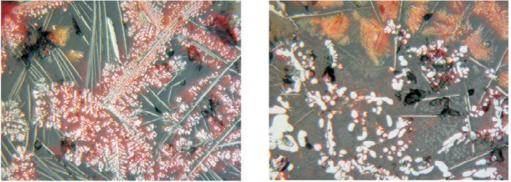
1, 2 – Pokrovskoe, sample 1311, 4th mineralogical group, length of the photo is 0.46 mm, crossed nicols: dendrites and deformed globules of cuprite and needles of delafossite.
