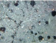
2 – sample 2032, 4th mineralogical group, 3rd type, Kelleli 4: long needles of olivine, small dendrites of cuprite (red fields), small grain and a prill of cuprite (white with blue tint), copper prills.
