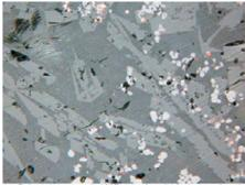
1 – Pokrovskoe, sample 1327, 1st mineralogical group, length of the photo is 0.02 mm: long skeletal crystals of fayalite (light grey) in the glass matrix (dark grey), small particles of magnetite (light) and small copper prills.
