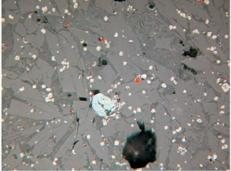
1 – sample 540, 1st mineralogical group, 2nd type Besh-Bulak 3: prismatic crystals of olivine (grey) in the glass matrix (dark grey), small needles and nuclei of olivine crystallization; octahedra of magnetite, small copper prills, fused grain of covellite (blue) and pores (black).
