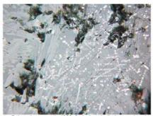
4 – Pokrovskoe, sample 1320, 2nd mineralogical group, length of the photo is 0.46 mm: crystals of olivine (light grey), dendrites of magnetite (light) and small prills of copper.
