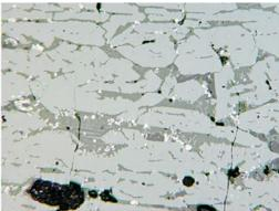
2 – prismatic crystals of fayalite (grey), very small octahedra of magnetite (white) and needles of fayalite in the glass matrix (dark grey).
