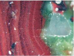
2 – Pokrovskoe, sample 1322, 4th mineralogical group, length of the photo is 0.62 mm, crossed nicols: strips from small prills of copper and cuprite, quartz grain with chrysocolla on the right
