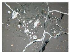
6 – Rodnikovskoye, sample 1332, 4th mineralogical group, length of the photo is 0.62 mm: small copper prills, Large cuprite globules and fillings of cracks.
