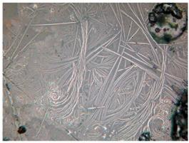
5,6 - sample 793, Kalinovka II - curved needles of delafossite, small copper prills and dendrites of magnetite in the glass matrix.
