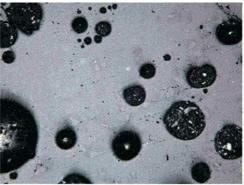
2 – Ostrovnoe III, sample 790 (length of the photo is 1.55 mm), small pores in the glass matrix.
