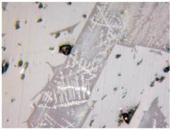
4 – Turbino I, sample 317 (length of the photo is 0.22 mm), polygonal crystals of olivine and small dendrites of magnetite.
