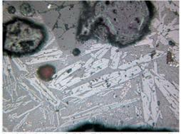
1 – skeletal prisms of olivine (light grey) and copper prills in the glass matrix (grey), quartz grain (dark grey above) with inclusion of a malachite grain and a particle of iron (length of the photo is 0.22 mm).
