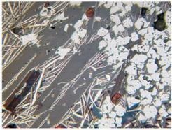
6 – Itkul I, sample 114 (length of the photo is 0.54 mm), octahedra of magnetite, needles of delafossite and copper prills in the glass matrix.
