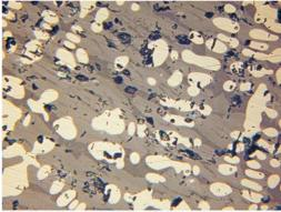
5 – Dolmatovo, sample 2033, fused dendrites of wüstite and prismatic crystals of fayalite.
