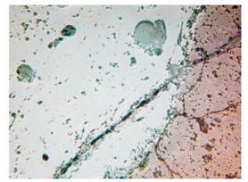
4 – sample 574, Besh-Bulak 4, accum. 2: upper part of slagged ceramic crust (pure glass, with inclusions of copper prills and grain of quartz on the left).
