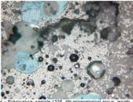
4 – Pokrovskoe, sample 1325, 4th mineralogical group, length of the photo is 0.62 mm: accumulation of magnetite particles keeping the form of a primary disintegrated grain, with inclusions of small copper prills. Grains of coveilite (blue) and malachite (grey-greenish on the left among the grains of coveilite), pores (black).
