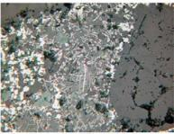
6 – Rodnikovskoye, sample 1347, 4th mineralogical group, I ength of the photo is 0.46 mm: quartz grain (dark grey on the right and on the left above), and particles, skeletons and dendrites of magnetite (light), and small grains of malachite (greenish).
