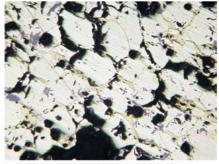
4 – Polished section of the roasted chalcopyrite. There is copper sulfide among the chalcopyrite grains, which explains easy crushing of these pieces.
