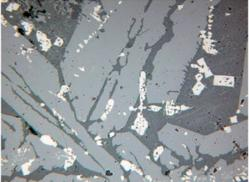
4 – large prisms of fayalite, skeletons of magnetite and dendrites of wüstite (white) and prisms of fayalite (grey).
