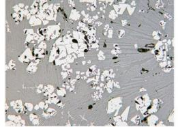
5 –large particles and small dendrites of magnetite (white), long skeletal crystals of olivine (light grey) in the glass matrix (grey) (length of the photo is 1.55 mm).
