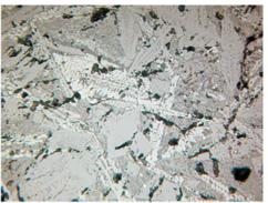
2 - Skorodum, sample 149 (length of the photo is 0.54 mm), prismatic crystals of olivine.
