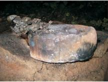
4 – Smelting bowl after operation. Only top part of its walls has actively contacted with molten slag, but the bowl can be used again.
