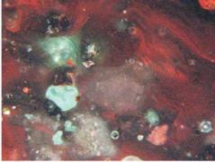
1 – Tokskoye, sample 1294, 4th mineralogical group, length of the photo is 0.62 mm, crossed nicols: strips from small prills of copper and cuprite painting slag in the red color, fine roundish grains of malachite and chrysocolla (green).
